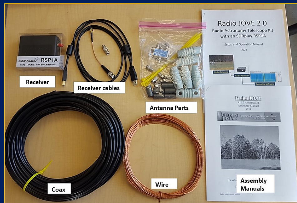
Radio JOVE 2.0 Hardware: SDRplay RSP1A, cables, Antenna Kit, assembly manuals, and Radio-Sky Spectrograph (RSS) software.
