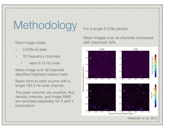
Each image is made using 5.079s of data imaged within 32 frequency channels, each 6.10 Hz wide. Initially, a mean image is made over all channels to identify the brightest meteor trails. For each of these detections, the antenna data are used to generate high-resolution(5.12ms) by beam forming to each source using a single 195.3 Hz wide channel.
