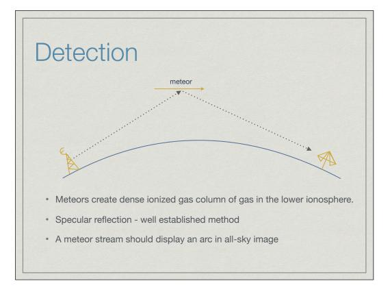
Meteors (as small as 10-5 g) entering the atmosphere create dense quasi-linear structures of ionized gas in the lower ionosphere (85 - 105 km high) during ablation 10s of km long.
