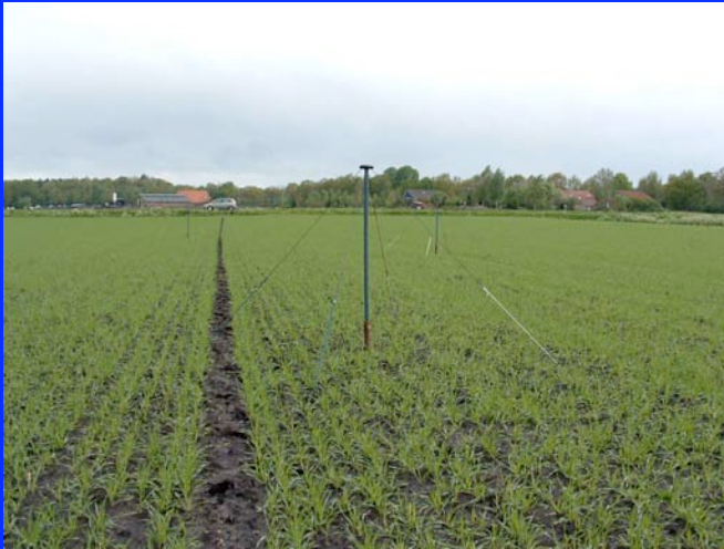
LOFAR low-band wire inverted-V
