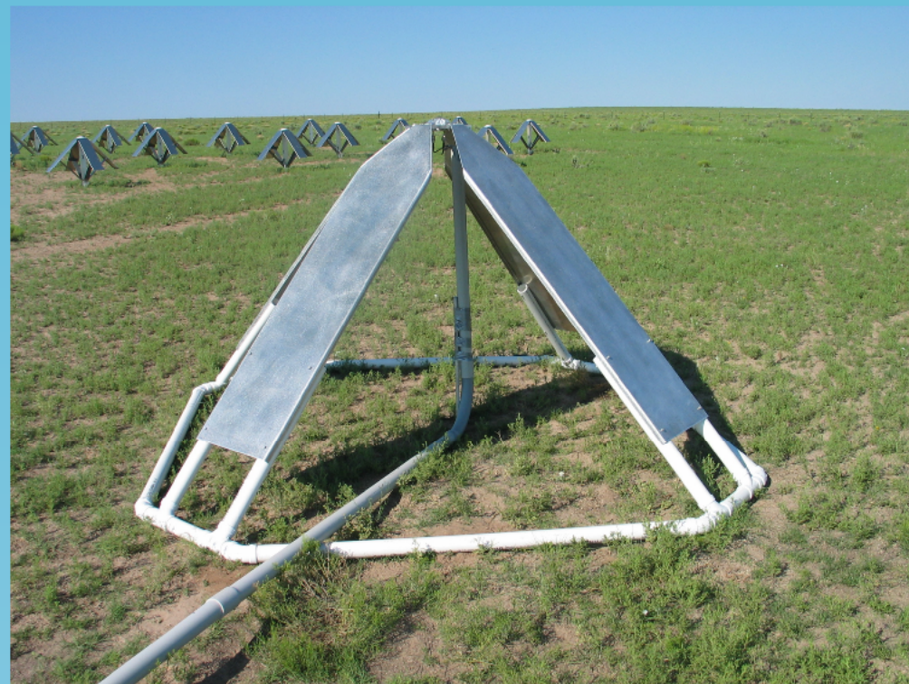
Photo of prototype "big blade" antenna. The full assembly of two dipoles and a mounting structure is referred to as a "stand".
