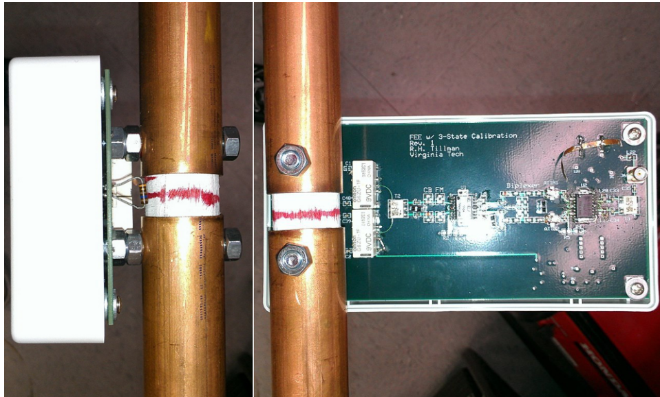
Figure 11: FEE integrated with the dipole antenna. Note: an older revision of the FEE is pictured (see appendix) but the interface has not changed.
