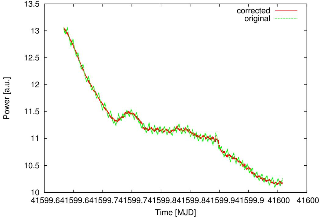
Figure 3: Example time variability of beam data for 42 MHz averaged over 1 MHz bandwidth for XX polarization pointing at zenith. The green line shows the original data, the red line is the data with the temperature variation measured by ASP subtracted.
