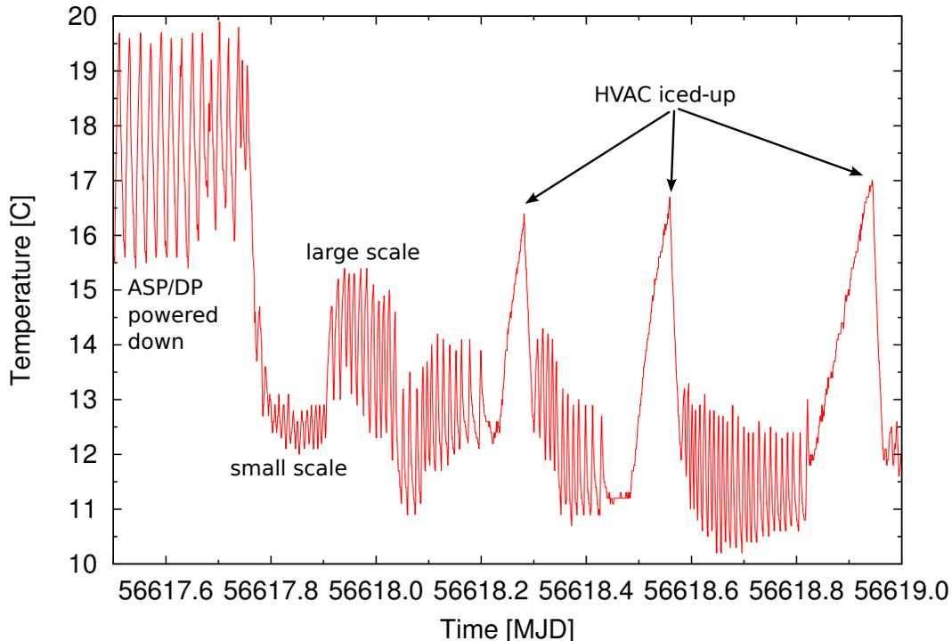
Figure 2: Example shelter temperature variation around November 22, 2013.
