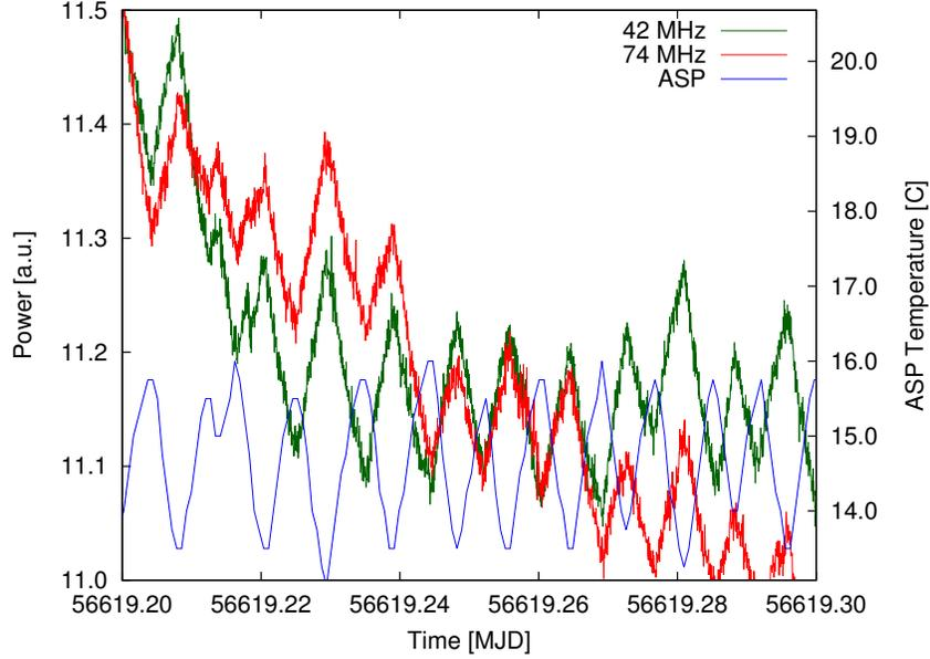
Figure 1: The blue curve, marked ASP, shows the temperature variations of the surface temperature of one of the ASP power supply units powering the frontend electronics. The red and green curves show the power level variation for the same stretch of time for XX polarization at 42 and 74 MHz pointing the beam at NCP.
