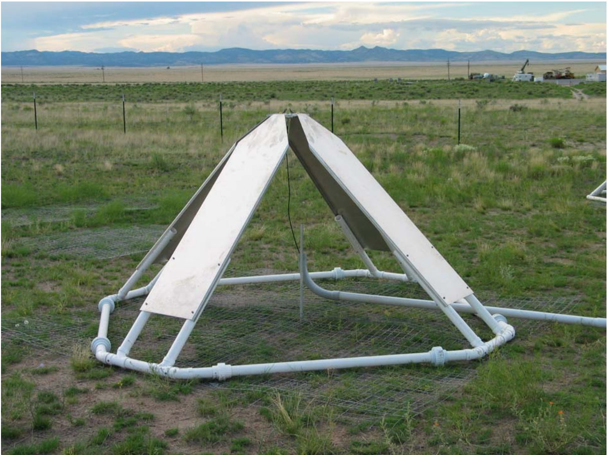
Fig. 1. A photograph of the Big Blade antenna over a ground screen.
