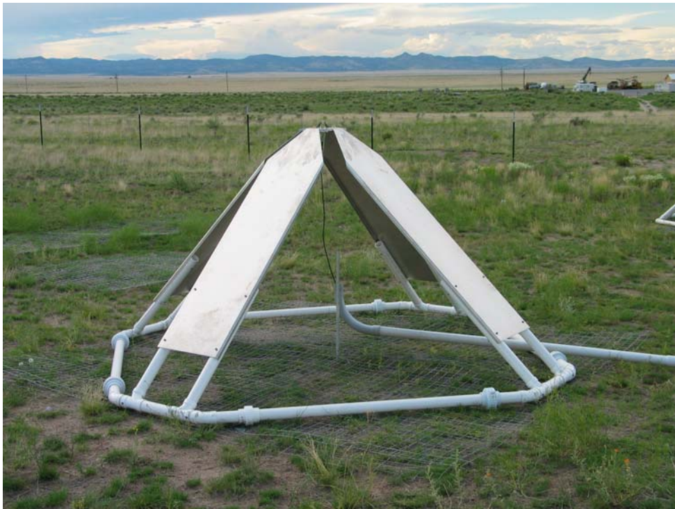
Fig. 41. A photograph of a big blade antenna prototype, modelled in Figure 40.
