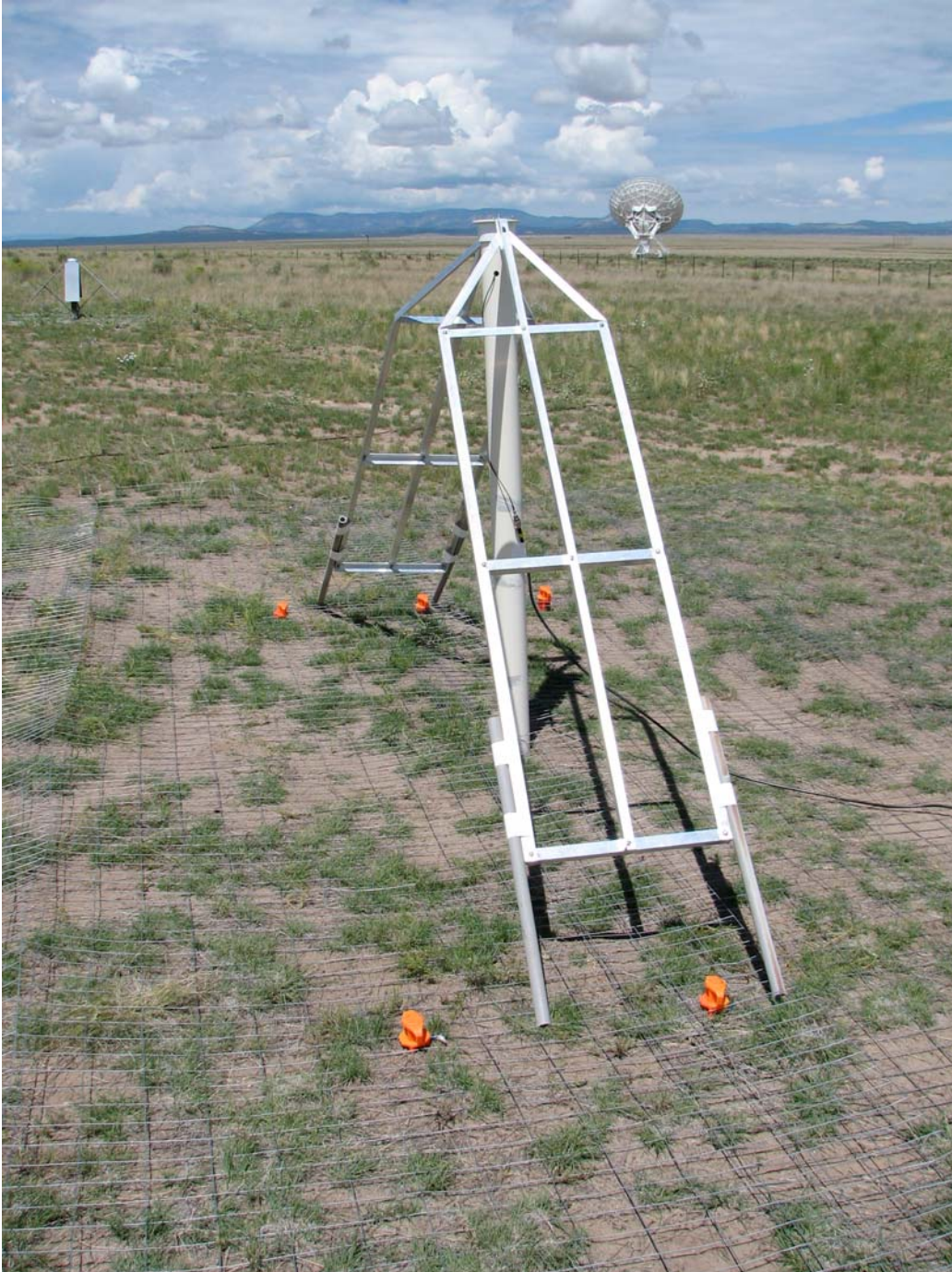
Fig. 2. A photograph of the Blade Frame antenna over a ground screen.
