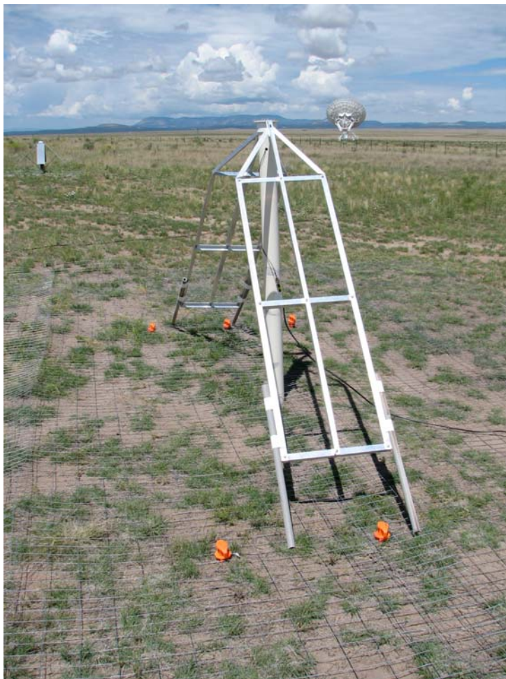
Fig. 18. A photograph of a Burns antenna prototype, modelled in Figure 17.
