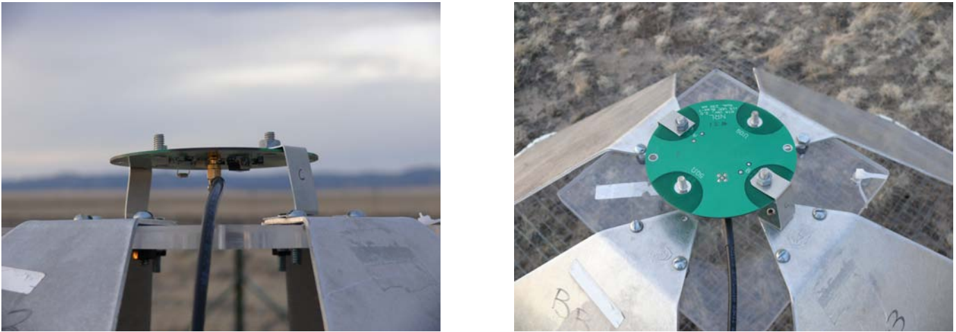
Fig. 6. The G250R balun mounted on a Big Blade antenna.
