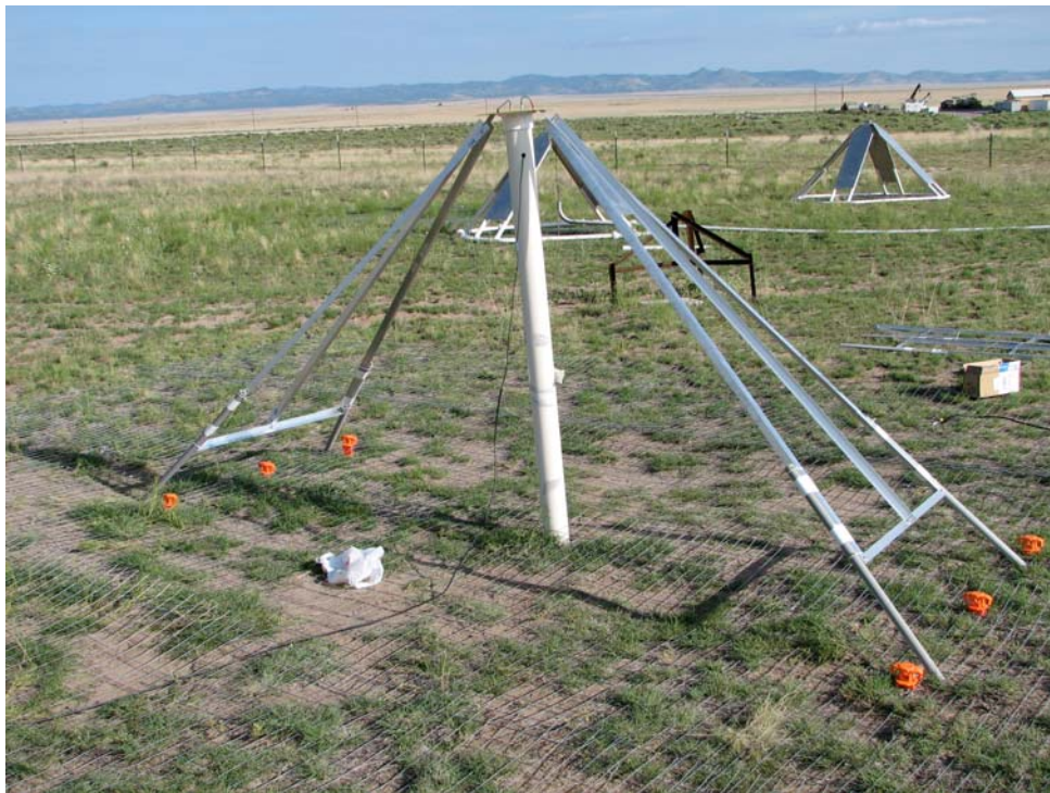
Fig. 26. A photograph a tied fork antenna prototype, modelled in Figure 25.
