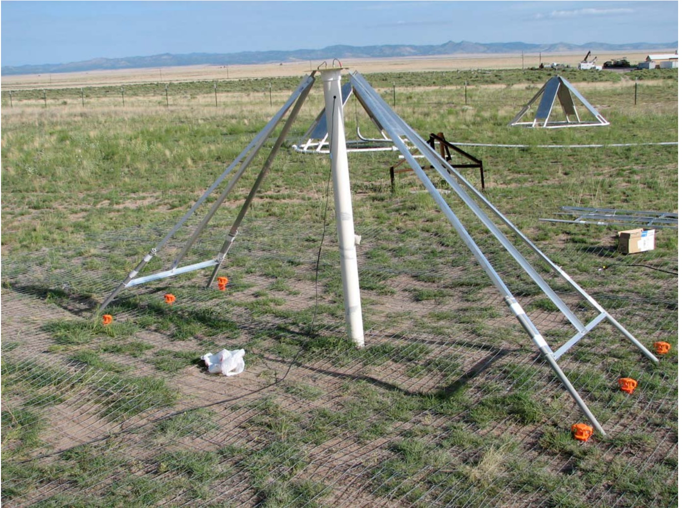
Fig. 3. A photograph of the Tied Fork antenna over a ground screen. Two versions of this antenna – one that was 1.5m long and one that was 1.7m long – were tested.
