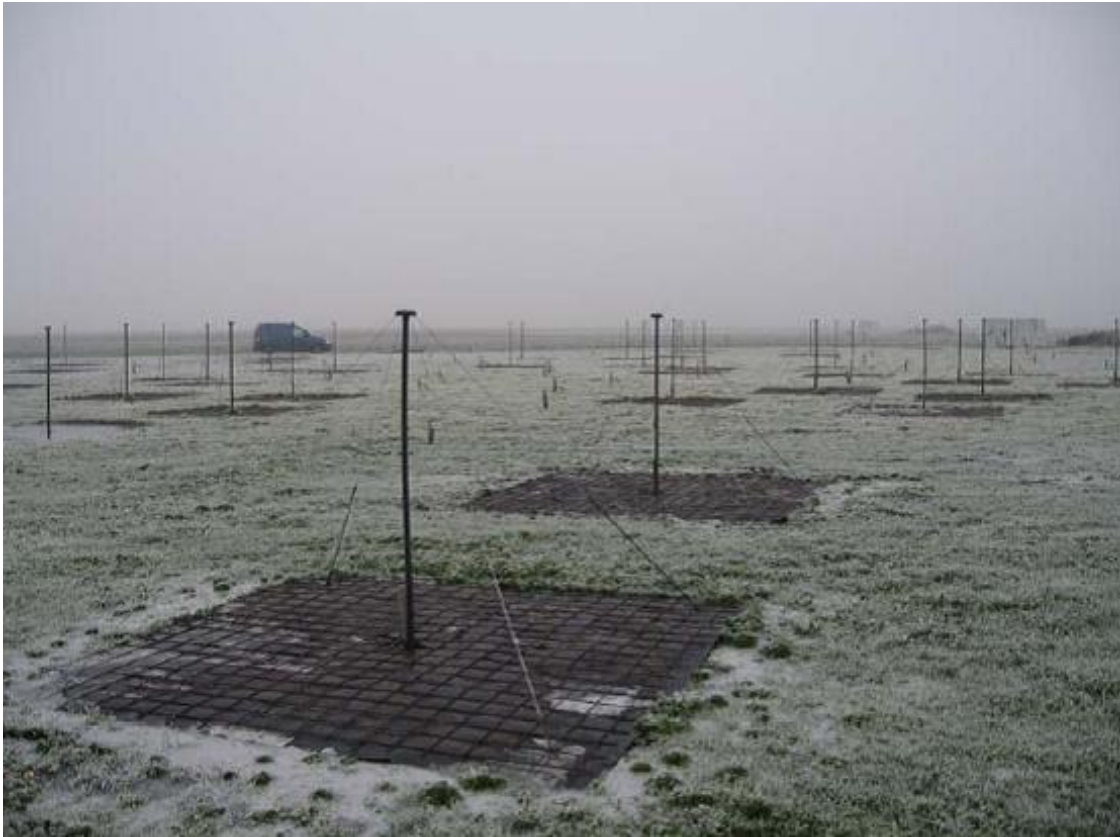
Fig. 2. A photograph of LOFAR low-band antennas similar to the inverted-V antenna modelled in Figure 1.
