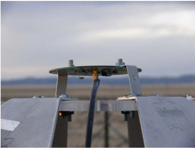
Fig. 6. The G250R balun mounted on a Big Blade antenna.
