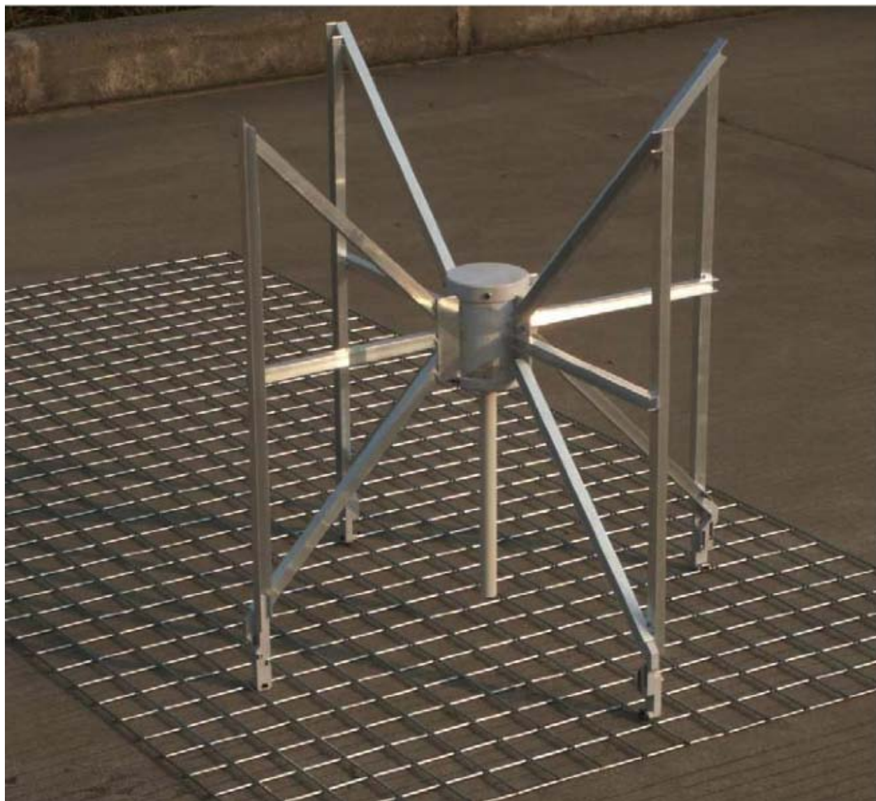
Fig. 10. A photograph of an MWA antenna. The bowtie antenna modelled in Figure 9 is this antenna scaled up in size by a factor of 3.
