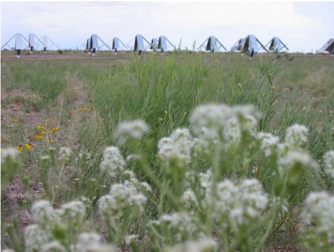
Figure 1. Photo of the Long Wavelength Demonstrator Array in New Mexico showing the individual dual-polarization stands. Each stand consists of four droopy blades which provide dual-polarization capabilities.
