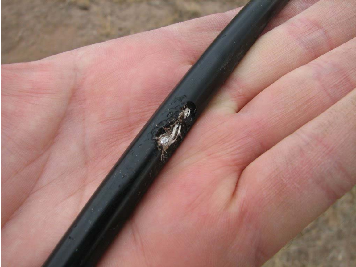
Figure 7: Another example of cable damage from animals.
