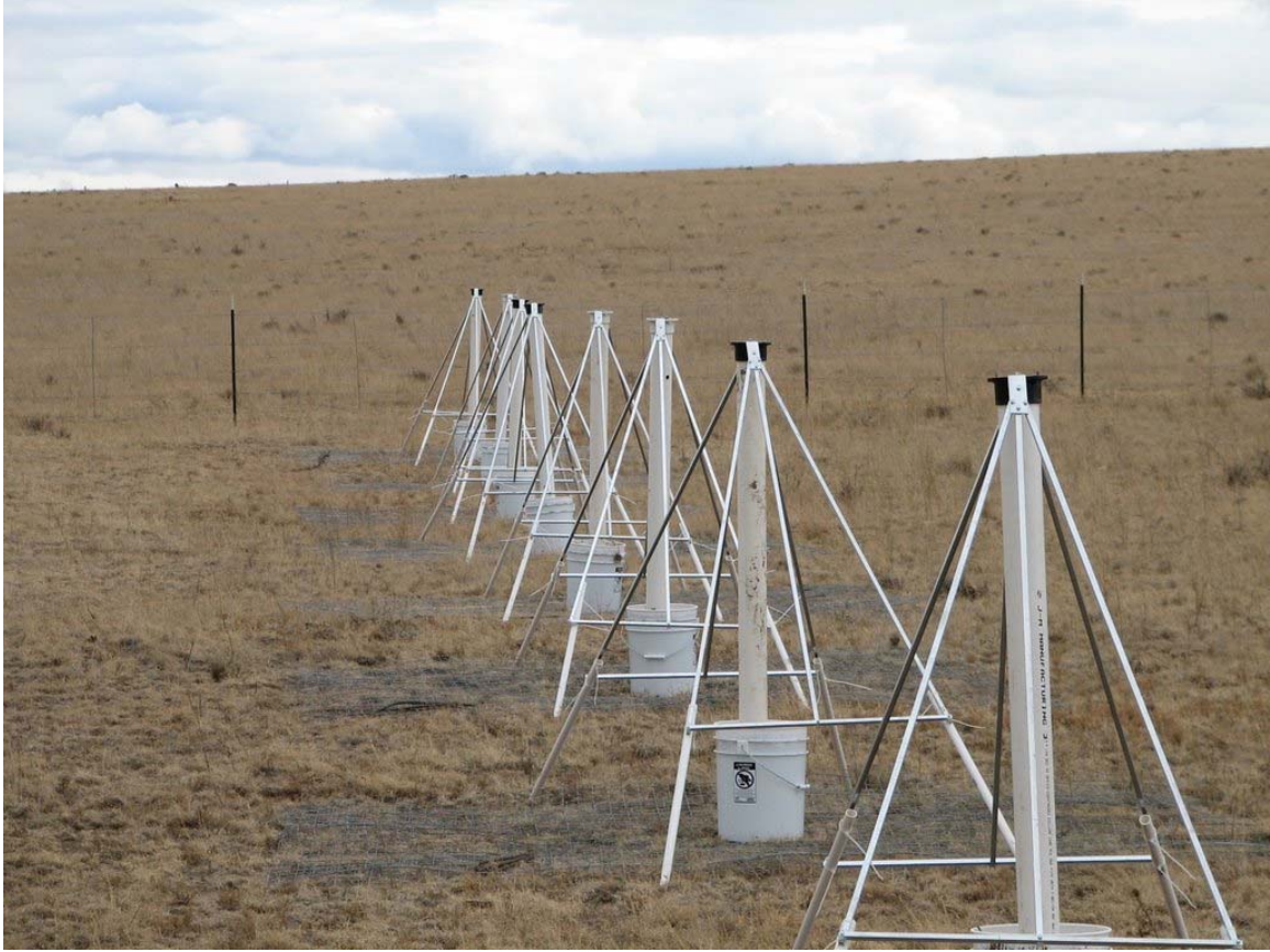
Figure 2: Single row of reconstructed and improved RTA-2 antennas. Unfortunately the improvised anchoring system using buckets of sand failed after a strong wind storm.
