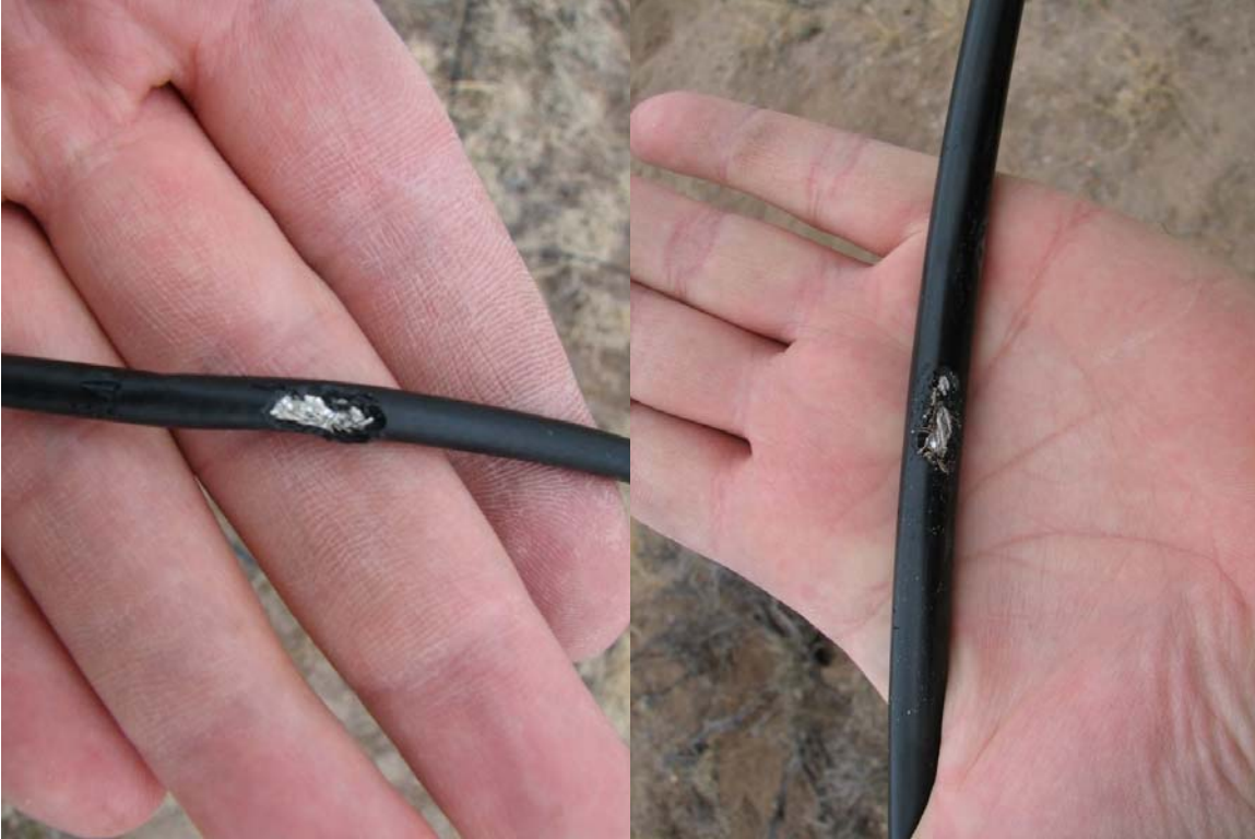
Figure 5 (left) and 6 (right): Examples of cable damage from animals.
