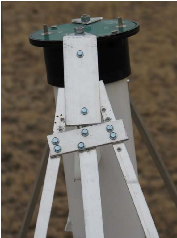
Figure 1: Example of inadequate RTA antenna construction.
