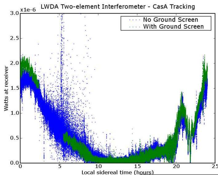
**Figure 8:** Power of received fringes from correlating the LWDA phased at CasA and the outlier dipole
