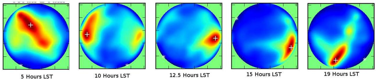
**Figure 6:** Spatial distribution of power at the times corresponding to inflection points of the signal level improvement for antenna 16
