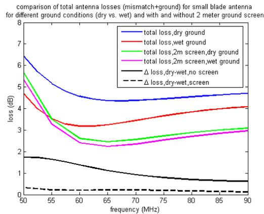
**Figure 2:** LWDA Ground Screen Simulation Results
