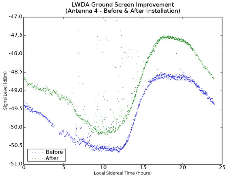
**Figure 4:** Antenna 4 power at receiver before and after ground screen installation
