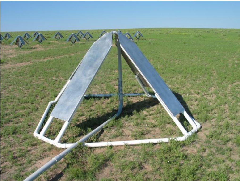
Fig. 7. A photograph of the dual polarization big blade antenna prototype (right), currently deployed at the LWDA site.
