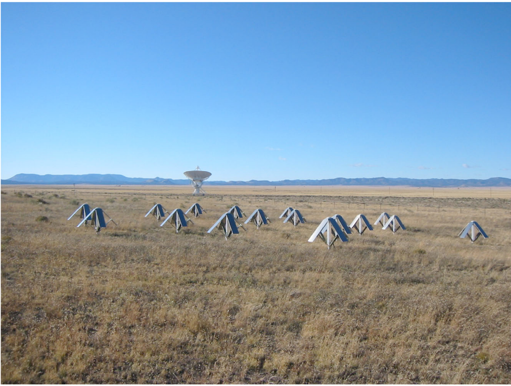
View of the 16 antennas on the LWDA site on the Plains of San Agustin in New Mexico with a 25-m VLA dish in the background.
