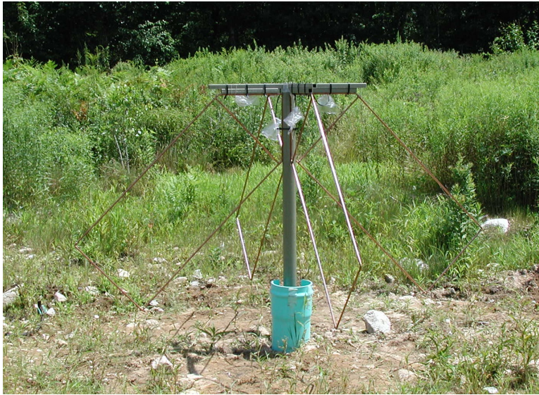
Fig. 2.— Photograph of GASE dipole installed at the Haystack Observatory site.
