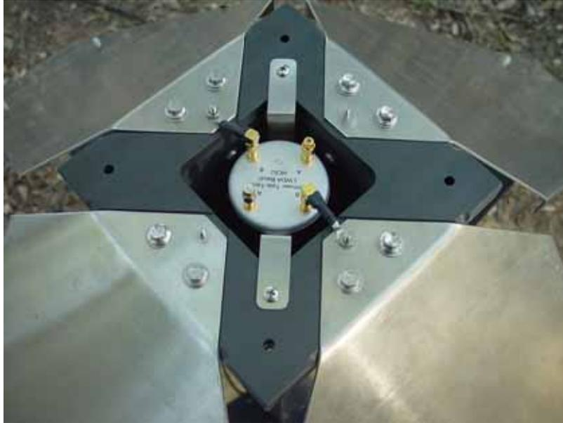
Figure 3. Top of antenna 1, showing the short cables antenna/balun cables.
