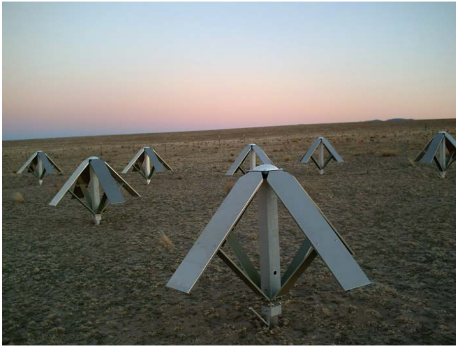
Fig. 1. A photograph of the small blade antennas at the LWDA site. There are currently a total of 16 of these antennas at the site.
