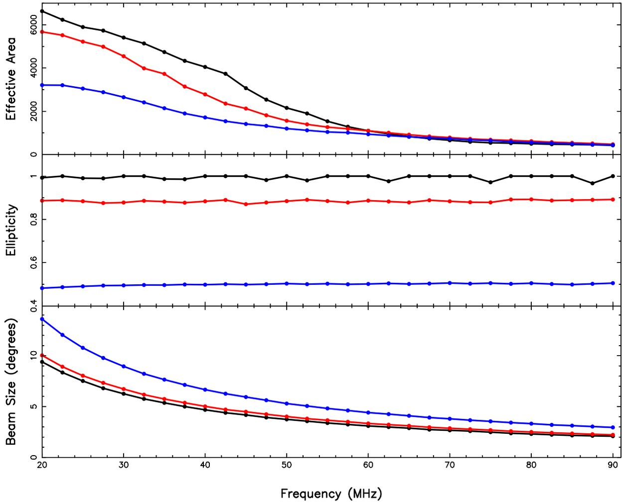
Fig. 6.— Strawman station effective area, beam ellipticity, and beam size as a function of frequency for three different zenith angles (black =  $0^\circ$ , red =  $30^\circ$ , blue= $60^\circ$ ). Element patterns have not been included in these metric calculations.
