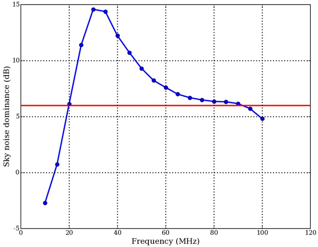
Fig. 4.— Simulated sky noise dominance (in dB; assuming a 250 K balun effective noise temperature and  $100 \Omega$  input impedance) as a function of frequency for the big blade antenna. The red line shows the LWA requirement of +6 dB. Values were computed using the impedance calculation from [CST Microwave Studio](#) assuming a perfect electrical conductor (PEC) ground, combined with Galactic noise model from [Cane \(1979\)](#).
