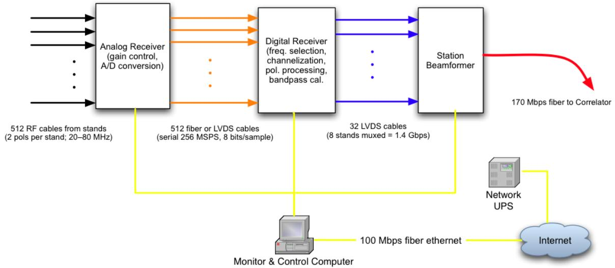
Fig. 9.— Block diagram of station electronics.
