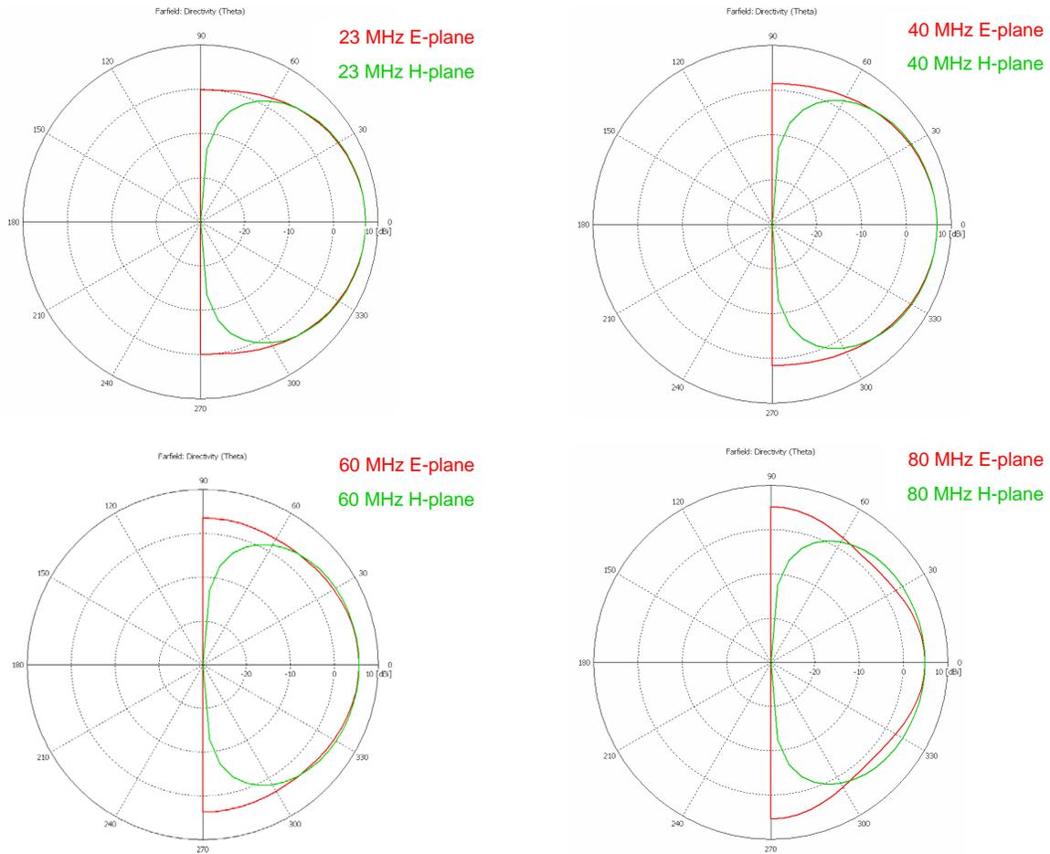
Fig. 3.— Simulated beam patterns (i.e. far-field directivity in dB) as a function of angle for the large blade antenna in both the E- and H-planes, for four different frequencies. Calculated using CST Microwave Studio assuming a perfect electrical conductor (PEC) ground.
