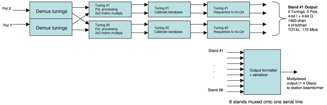
Fig. 12.— Digital receiver block diagram, second section.
