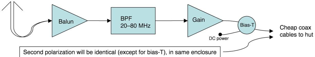
Fig. 8.— Front end electronics block diagram.
