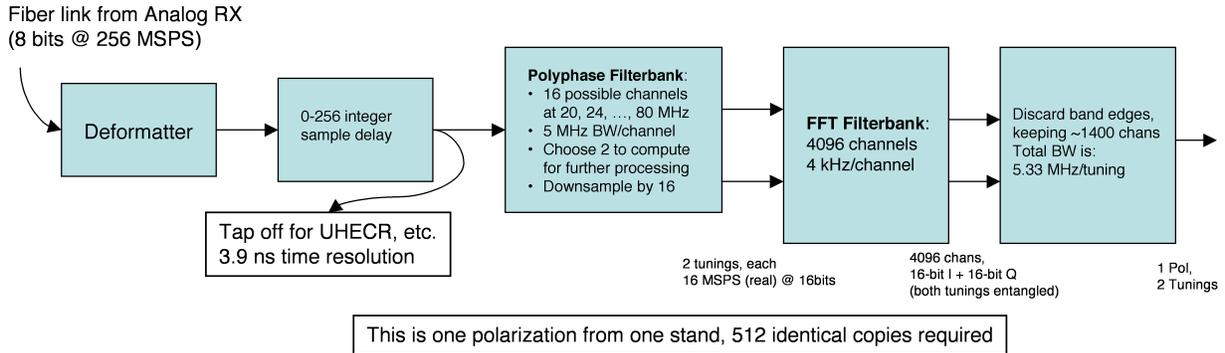
Fig. 11.— Digital receiver block diagram, first section.
