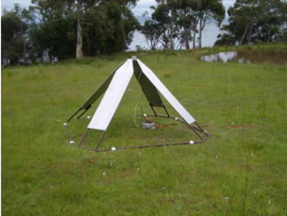
Fig. 1.— Strawman big blade antenna on a PVC pyramidal mount.
