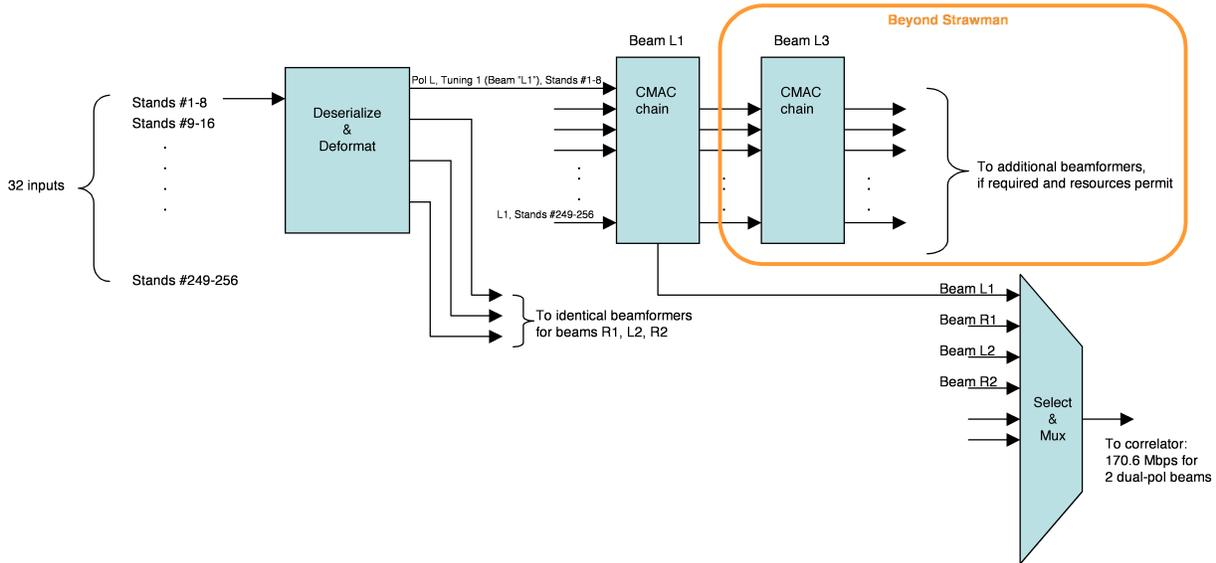
Fig. 13.— Beamformer block diagram.
