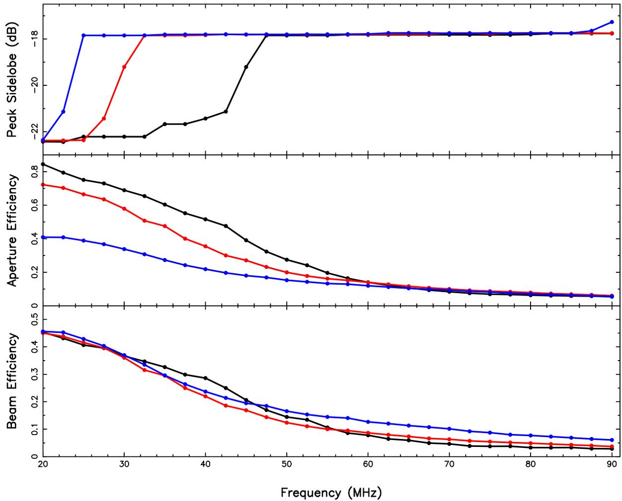
Fig. 7.— Strawman station peak sidelobe level, aperture efficiency, and beam efficiency as a function of frequency for three different zenith angles (black =  $0^\circ$ , red =  $30^\circ$ , blue =  $60^\circ$ ). Element patterns have not been included in these metric calculations.
