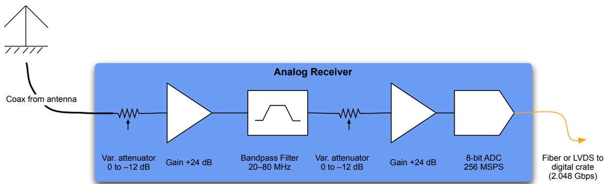
Fig. 10.— Analog receiver block diagram. This shows a single analog chain (one polarization from one stand) out of the 512 needed for a full station.
