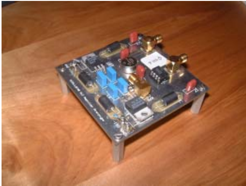
Active-balun prototype utilizing commercial wide-bandwidth Operational Amplifier
