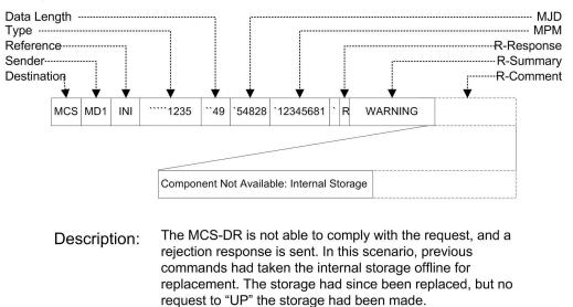
Figure 4: Example of requesting initialization (w/Error Response)
