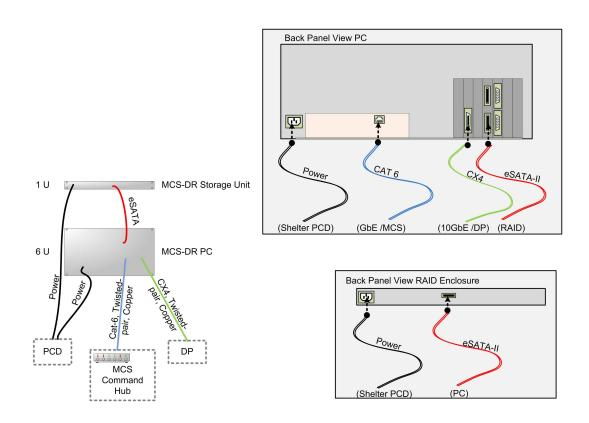
Figure 2: Diagram of electrical connections
