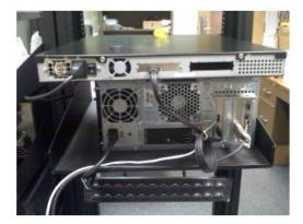
Figure 1: An MCS-DR PC and storage unit mounted on a 19" rack
