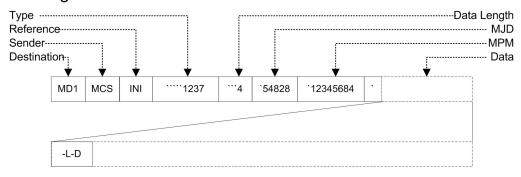
Description: MCS requests initialization of the system with the "-L" and "-D" options. The options specified request that the MCS-DR clear its internal log and any previously recorded data.
