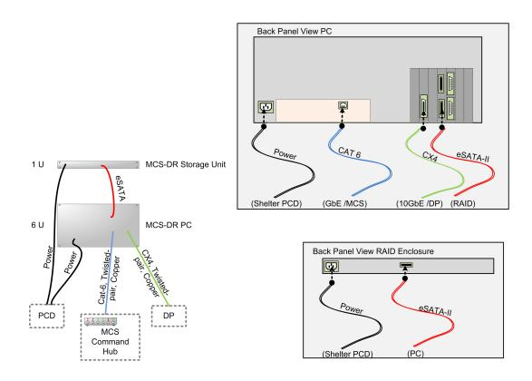
Figure 2: Diagram of electrical connections
