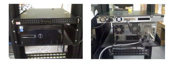
Figure 1: An MCS-DR PC and storage unit mounted on a 19" rack
