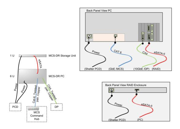
Figure 2: Diagram of electrical connections
