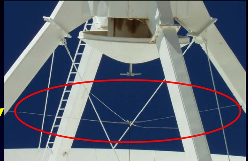
Crossed dipole suspended below sub-reflector by wires
