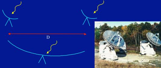
Consider two dishes with separation  $D$  vs. one dish of diameter  $D$ . By combining the radio waves from the two dishes, the achieved angular resolution is the same as the large dish.
