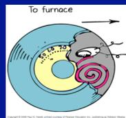
The unequal expansion of a bimetallic strip can operate a thermostat.
