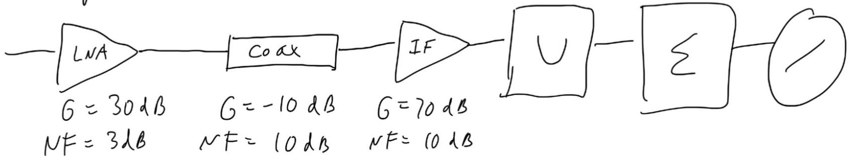
$$NF = \frac{T_{noise}}{T_{ref}} + 1 \quad T_{ref} = 290 \text{ K}$$
