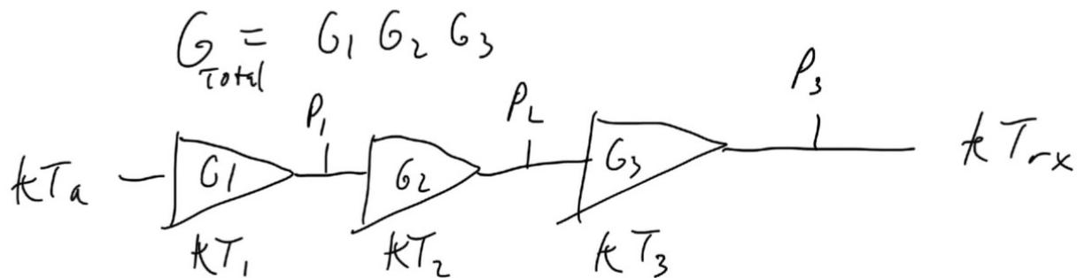
$$P_1 = (kT_a + kT_1) G_1 \quad \text{and} \quad P_3 = k(T_a + T_{rx}) G_1 G_2 G_3$$
