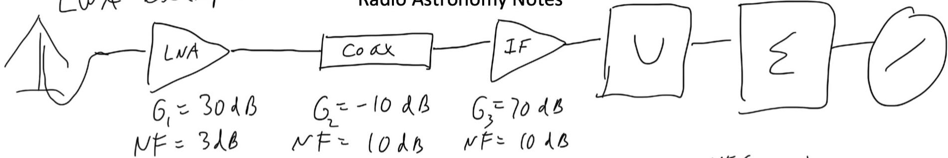
$$NF = \frac{T_{noise}}{T_{ref}} + 1 \quad T_{ref} = 290 K \quad T = T_{ref} (10^{NF/10} - 1)$$
