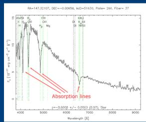
For a gas of a given element, absorption and emission lines occur at same wavelengths.
