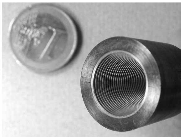
Fig. 7.5 A corrugated waveguide hybrid mode feed for \lambda 2 mm for the IRAM Plateau de Bure interferometer (courtesy of B. Lazareff)
