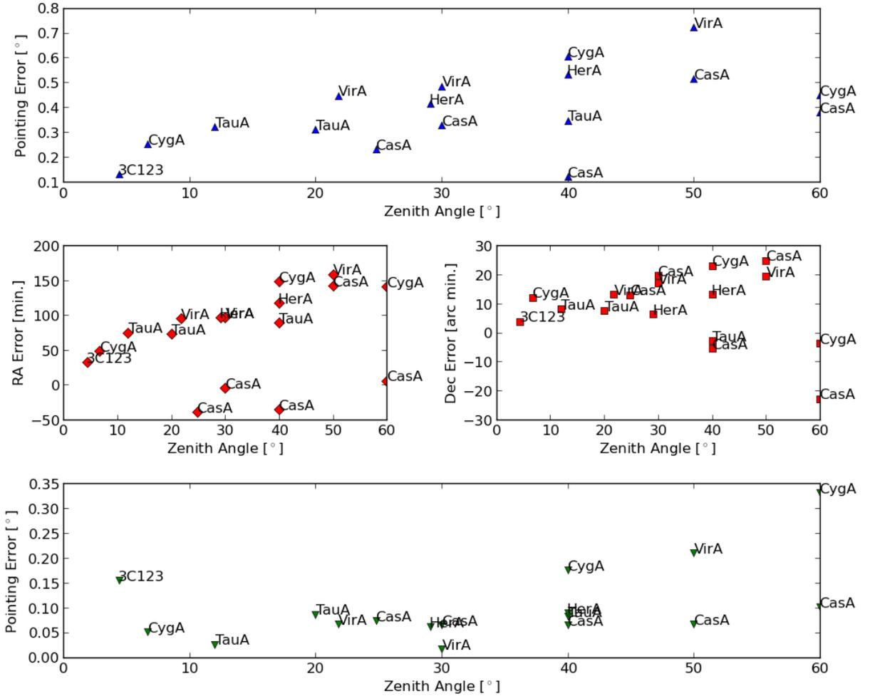
Figure 3: Comparison between the raw pointing offsets (total – top panel; by RA and Dec. – middle two panels) and the corrected pointing offsets (bottom panel). The source associated with each data point is listed to the upper right. Before correction the mean pointing error is  $\sim 0.4^\circ$  and the mean error is  $\sim 0.1^\circ$  after correction.
