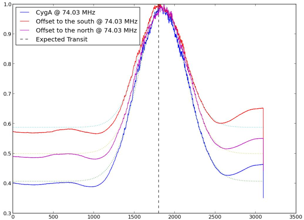
Figure 2: Plot of the spectrometer data collected for the Cyg A run on March 6, 2013. The x-axis is in UTC time while the y-axis is in linear power. The best-fit Gaussians for each of the beams are plotted as dashed lines while the beam transit times determined from the Gaussian fits are plotted as dotted lines. For this data, the error in RA is  $\sim 1$  minute and the error in declination is  $\sim 13'$ .
