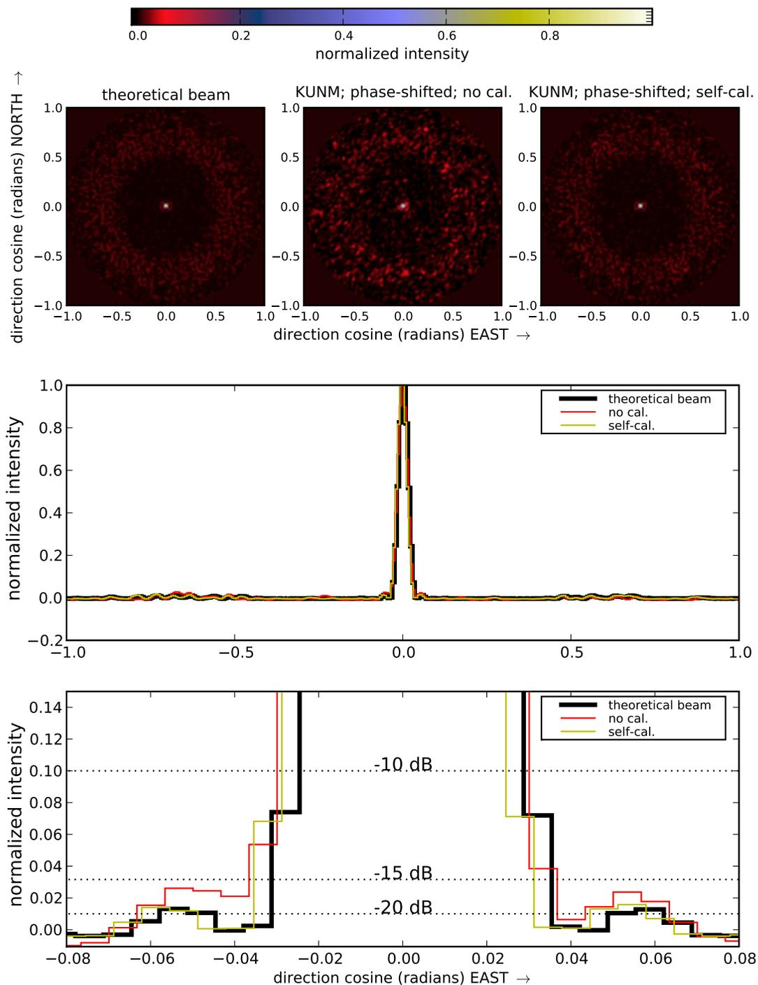
Figure 1: Upper: At 89.9 MHz the theoretical beam (left), a phase-shifted image of the KUNM transmitter (middle), and an image of the transmitter after self-calibration (right). Middle: East-west slices through the brightest pixels in the three images shown above. Lower: The same as the middle panel, but zoomed in to show the first sidelobes.
