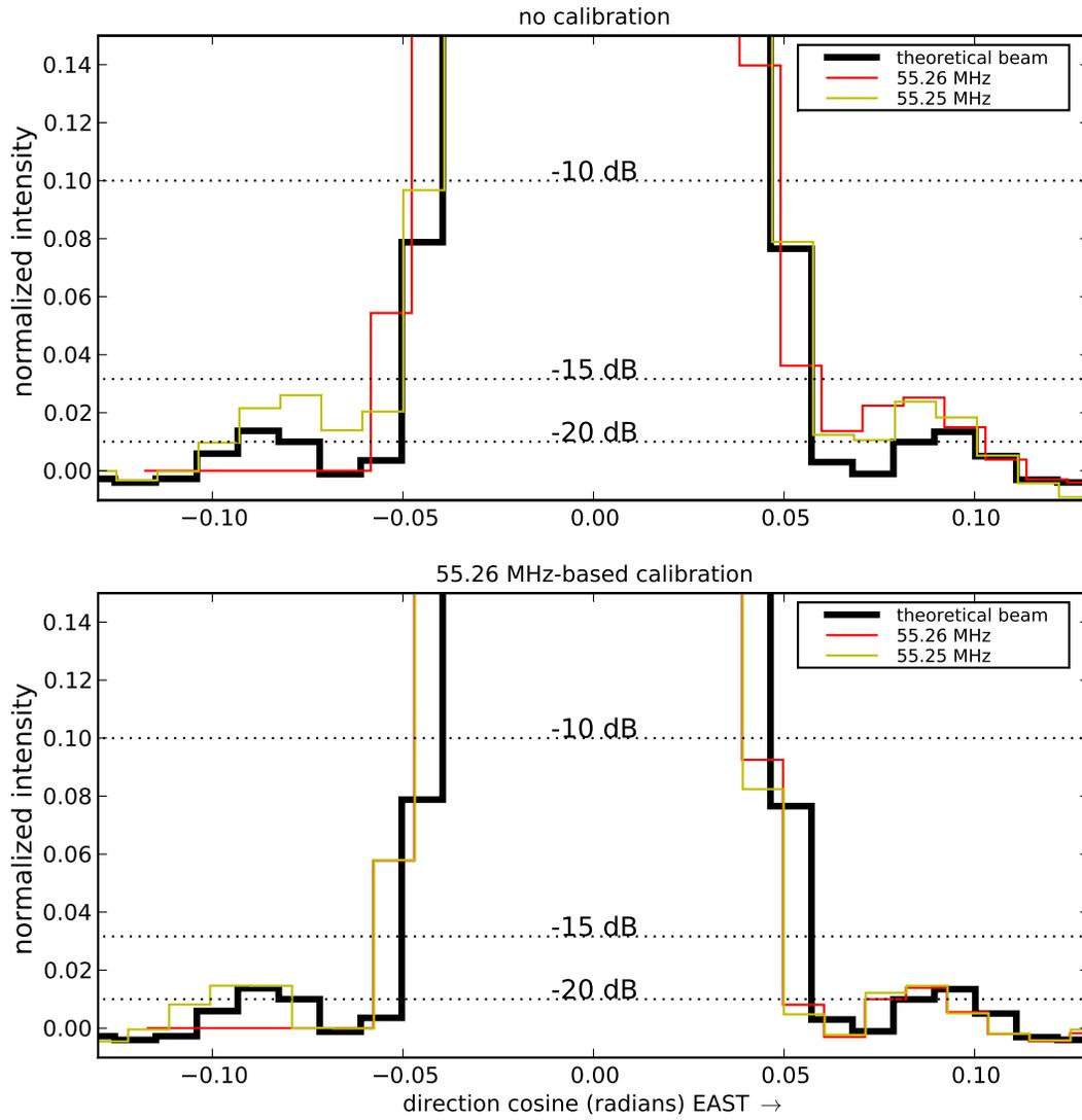
Figure 3: East-west slices through the brightest pixels in the images shown in Fig. 2 as well as the theoretical beam before (upper) and after (lower) self-calibration.
