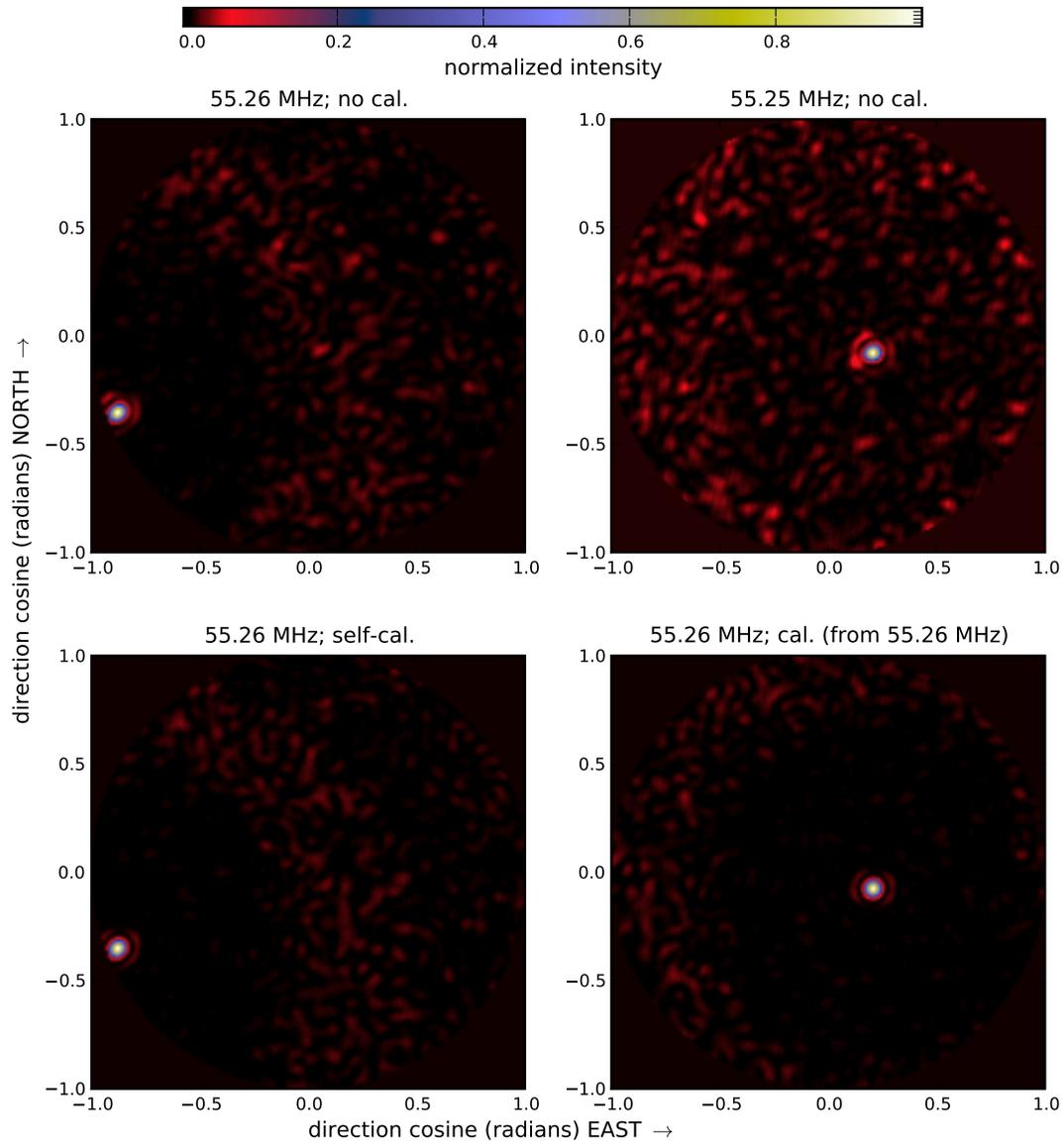
Figure 2: Images of echoes at 55.26 MHz (left) and 55.25 MHz (right) before (upper) and after (lower) applying gain corrections derived from performing self-calibration with the 55.26 MHz echo.
