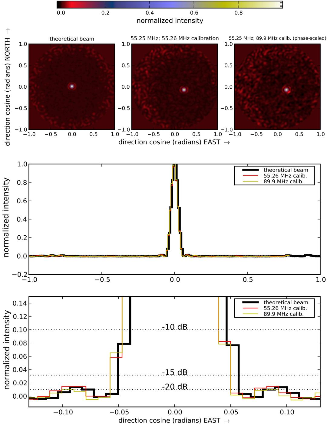
Figure 5: Upper: The theoretical 55.25 MHz beam (left), the 55.25 MHz echo calibrated with the 55.26 MHz gains (middle) and the same calibrate with the 89.9 MHz gains. East-west slices through the peak pixels of these three images are shown in the lower two panels.
