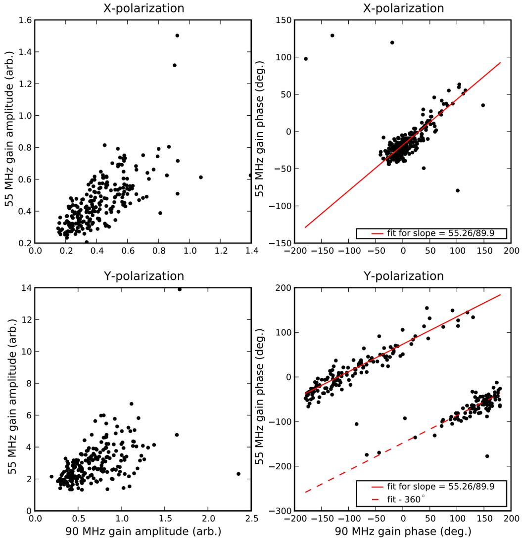
Figure 4: The amplitude (left) and phase (right) of the 55.26 MHz gains versus those determined at 89.9 MHz for the X (upper) and Y (lower) polarizations. In the right panels, the red lines show the expected relationship if the phases simply scale with frequency (i.e., a line with a slope of 55.26/89.9).
