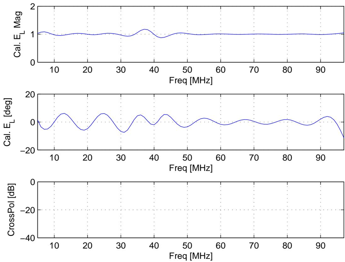
Figure 18:  $\theta = 0$  (zenith),  $\phi = 0$ : Calibrated LCP using  $M = 16$  taps. Maximum tap dynamic range is 32 dB. Crosspol in this case is effectively perfect (limited only by numerical precision).
