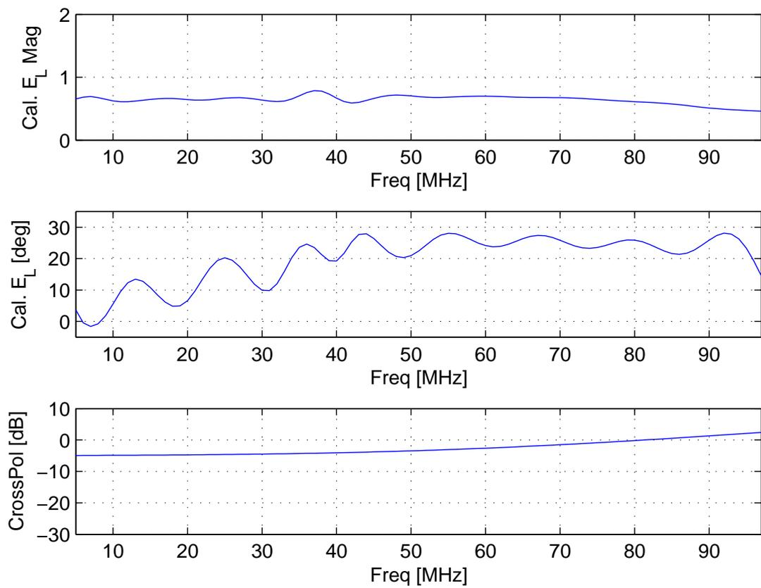
Figure 23:  $\theta = 74^\circ$ ,  $\phi = 0$ : Calibrated LCP using  $M = 16$  tap solution for  $\theta = 0^\circ$ . *Note modified scales in lower two plots.*
