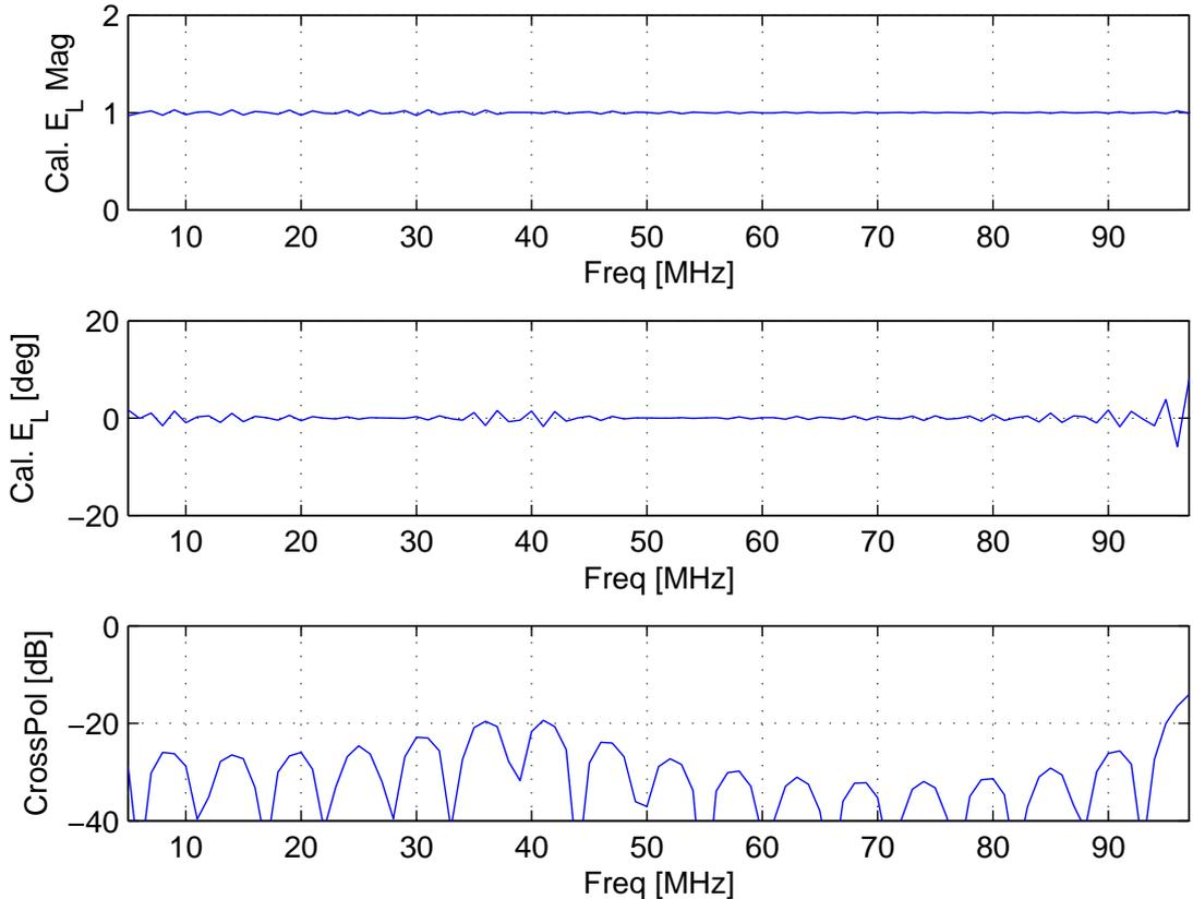
Figure 12:  $\theta = 74^\circ$ ,  $\phi = 45^\circ$ : Calibrated LCP using  $M = 80$  taps. Maximum tap dynamic range is 41 dB.
