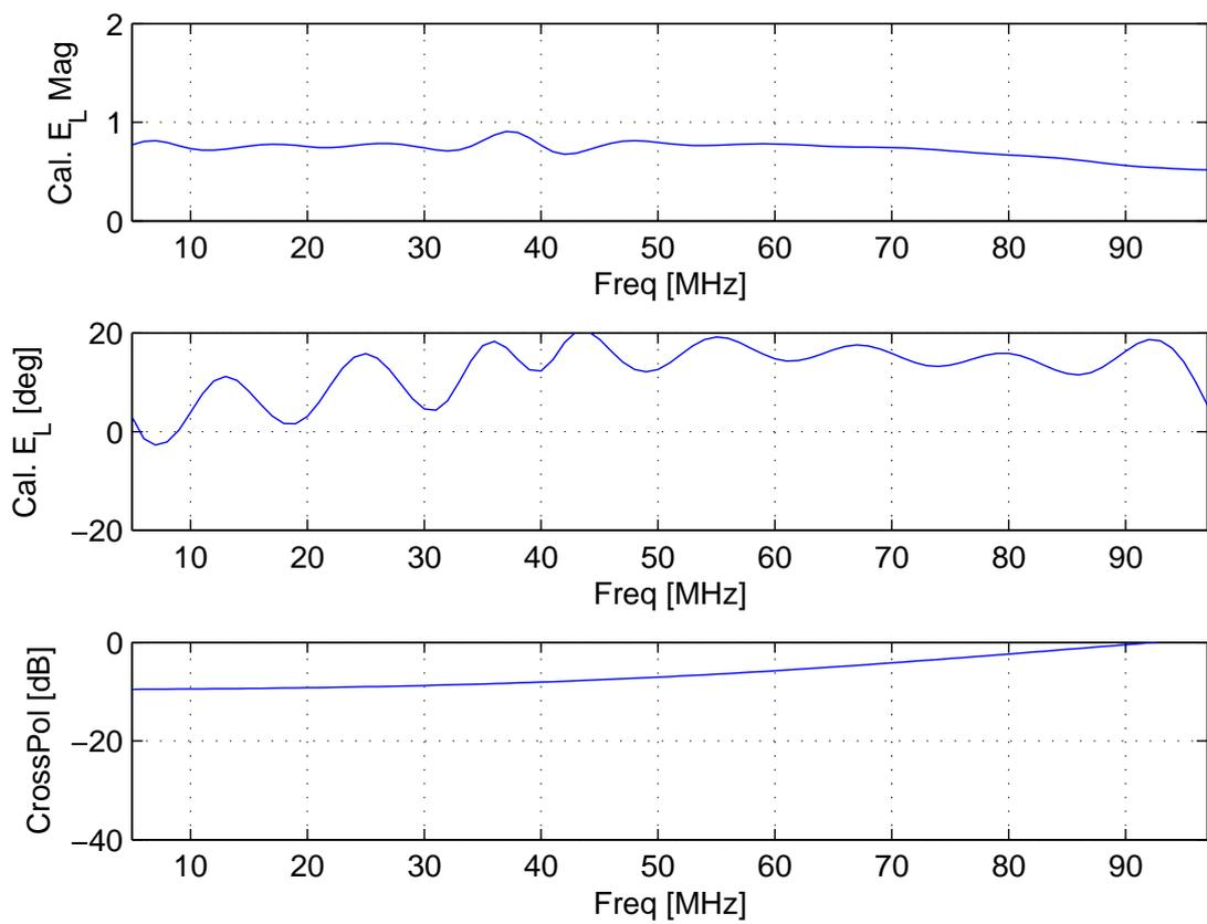
Figure 22:  $\theta = 60^\circ$ ,  $\phi = 0$ : Calibrated LCP using  $M = 16$  tap solution for  $\theta = 0^\circ$ .
