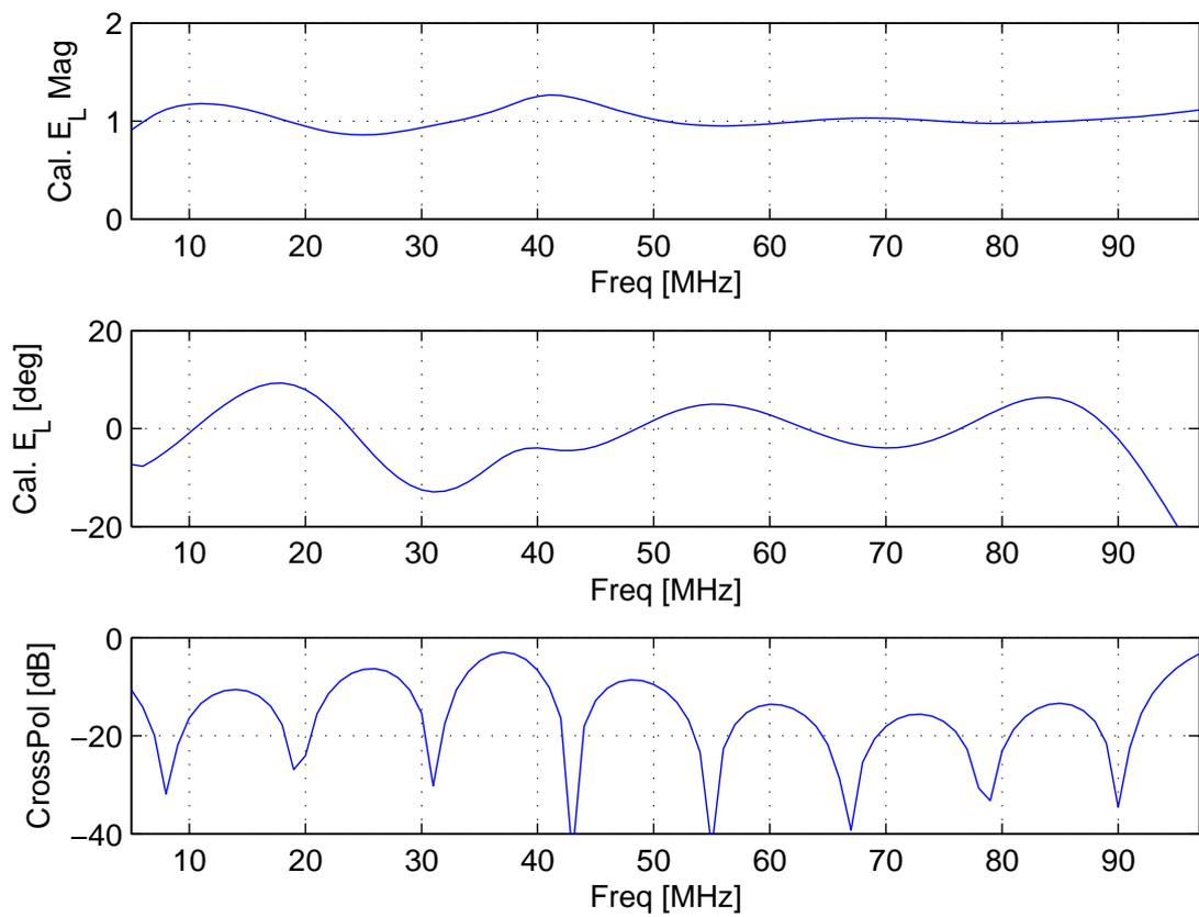
Figure 15:  $\theta = 74^\circ$ ,  $\phi = 45^\circ$ : Calibrated LCP using  $M = 8$  taps. Maximum tap dynamic range is 23 dB.
