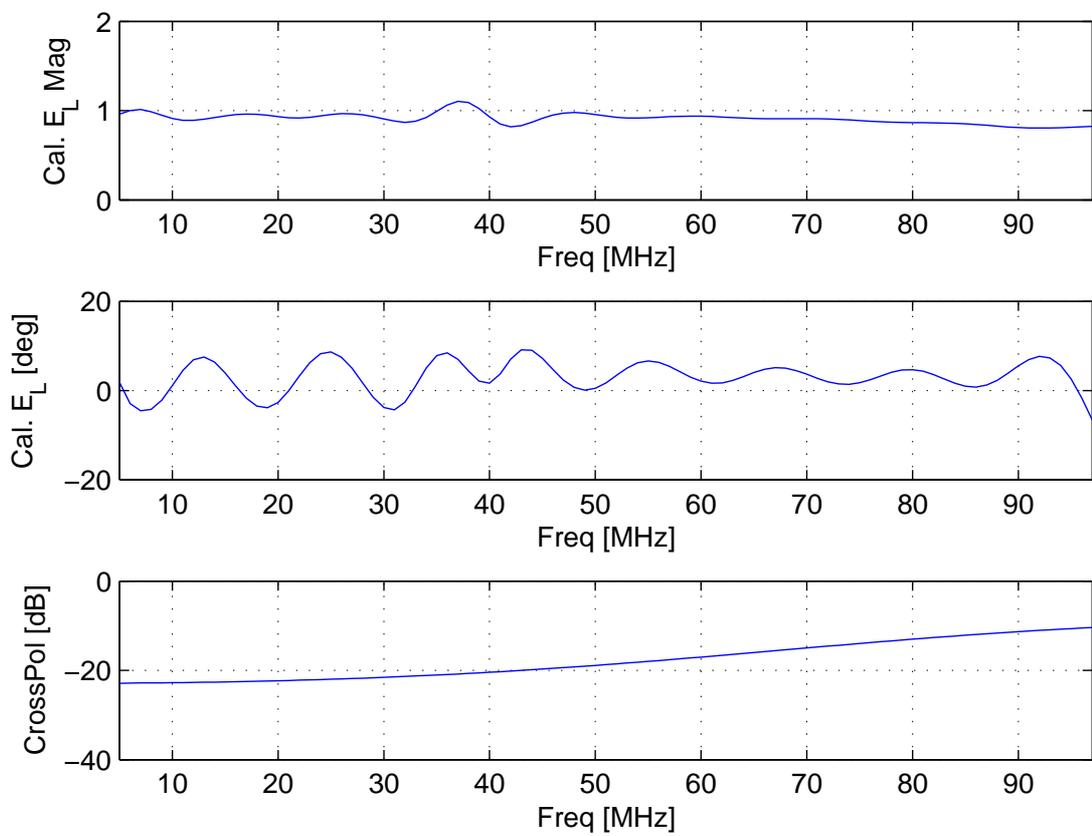
Figure 20:  $\theta = 30^\circ$ ,  $\phi = 0$ : Calibrated LCP using  $M = 16$  tap solution for  $\theta = 0^\circ$ .
