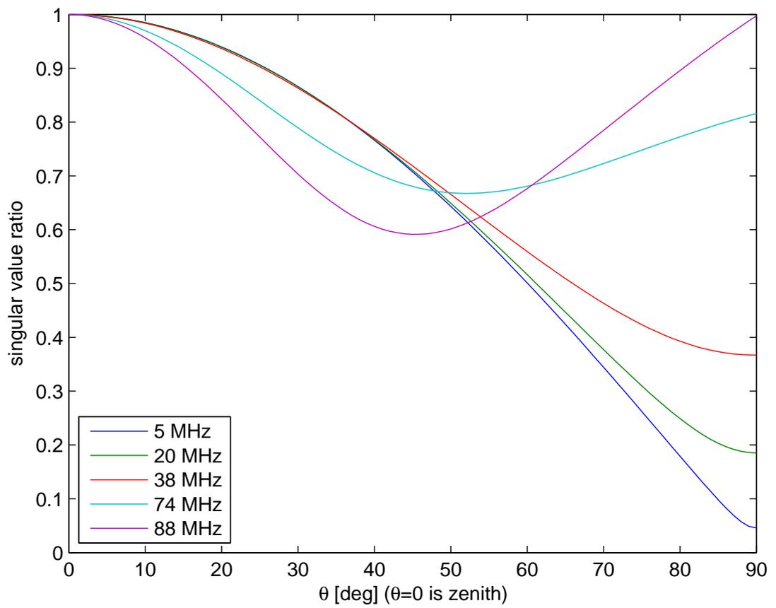
Figure 10: Efficacy of polarization calibration expressed in terms of singular value ratio; larger is better.  $\phi = 0$ .
