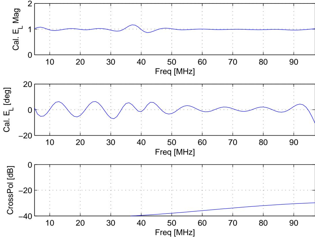
Figure 19:  $\theta = 10^\circ$ ,  $\phi = 0$ : Calibrated LCP using  $M = 16$  tap solution for  $\theta = 0^\circ$ .
