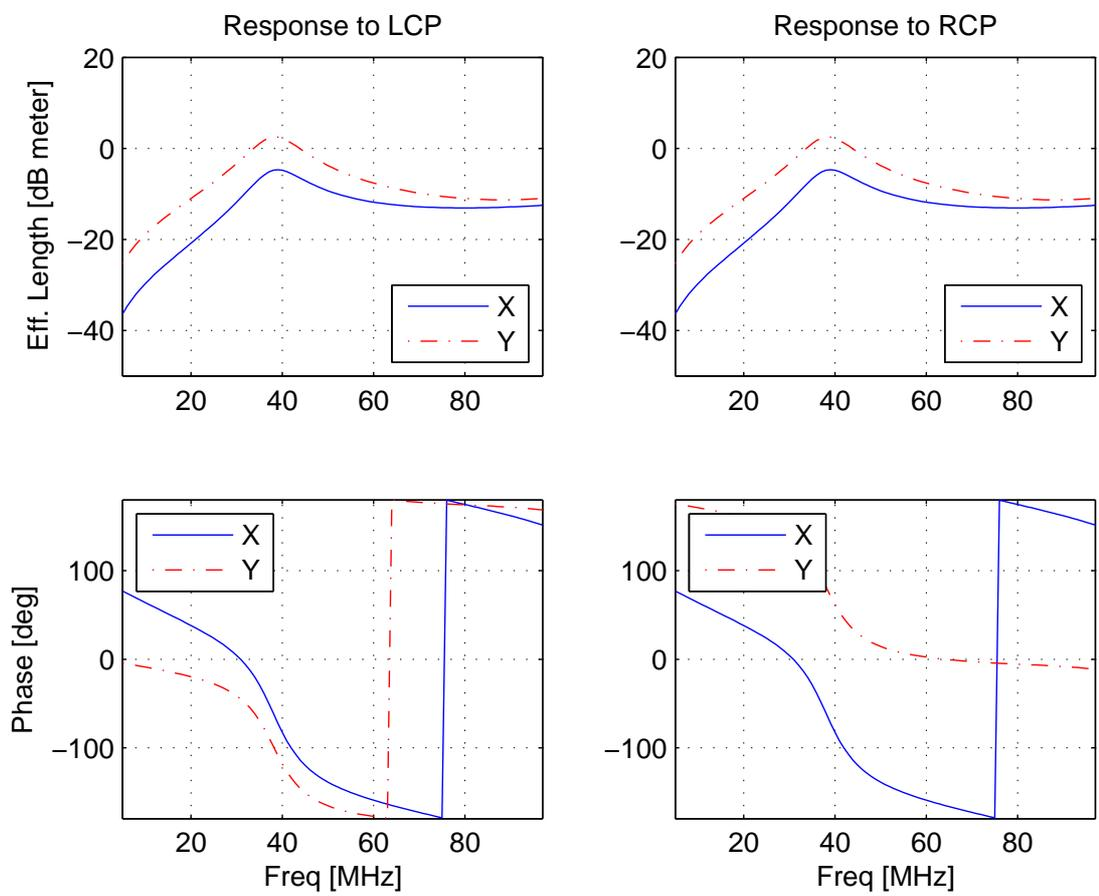
Figure 5:  $\theta = 74^\circ$ ,  $\phi = 0$ : Active balun input.
