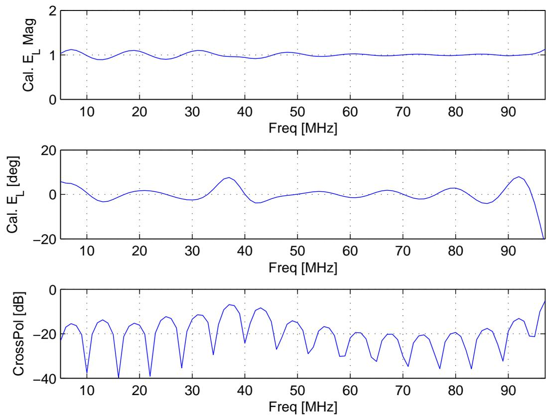
Figure 14:  $\theta = 74^\circ$ ,  $\phi = 45^\circ$ : Calibrated LCP using  $M = 16$  taps. Maximum tap dynamic range is 29 dB.
