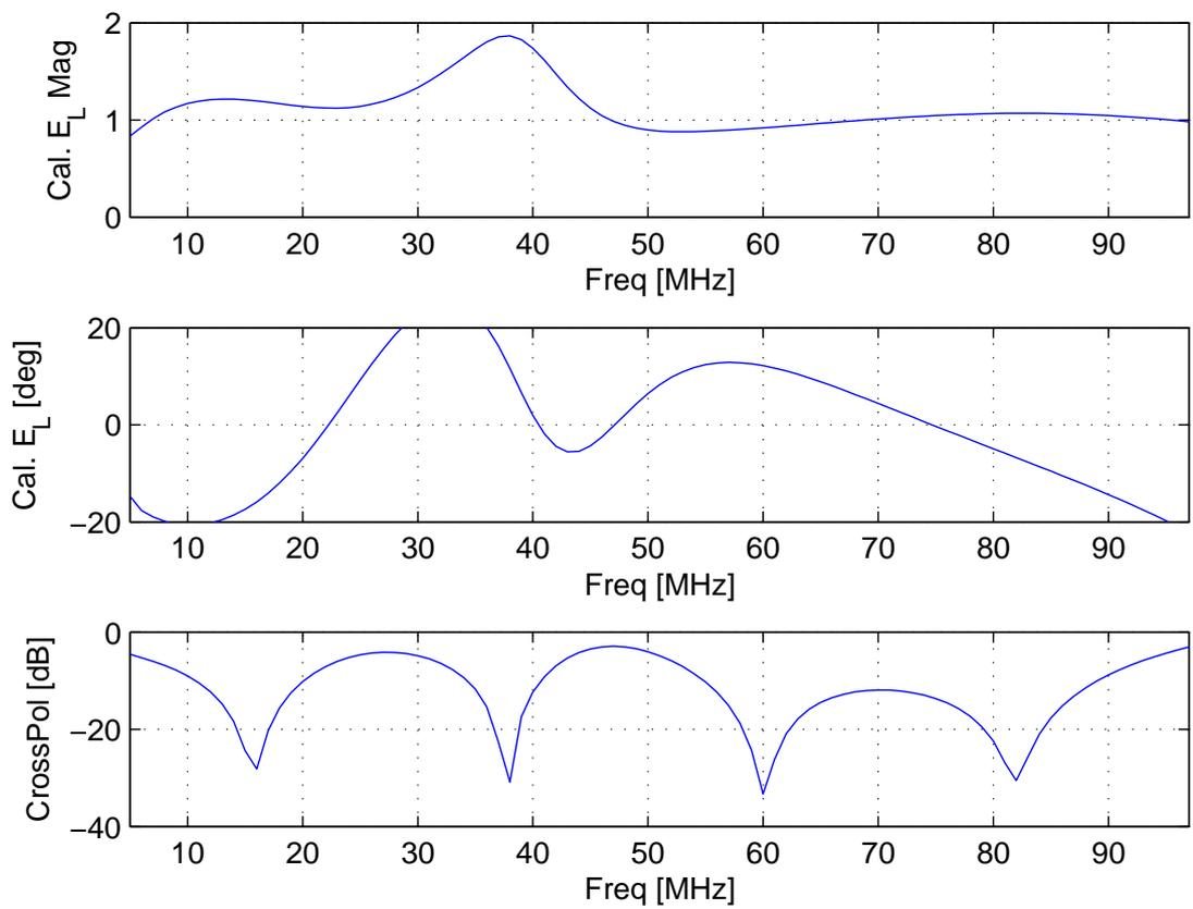
Figure 16:  $\theta = 74^\circ$ ,  $\phi = 45^\circ$ : Calibrated LCP using  $M = 4$  taps. Maximum tap dynamic range is 14 dB.
