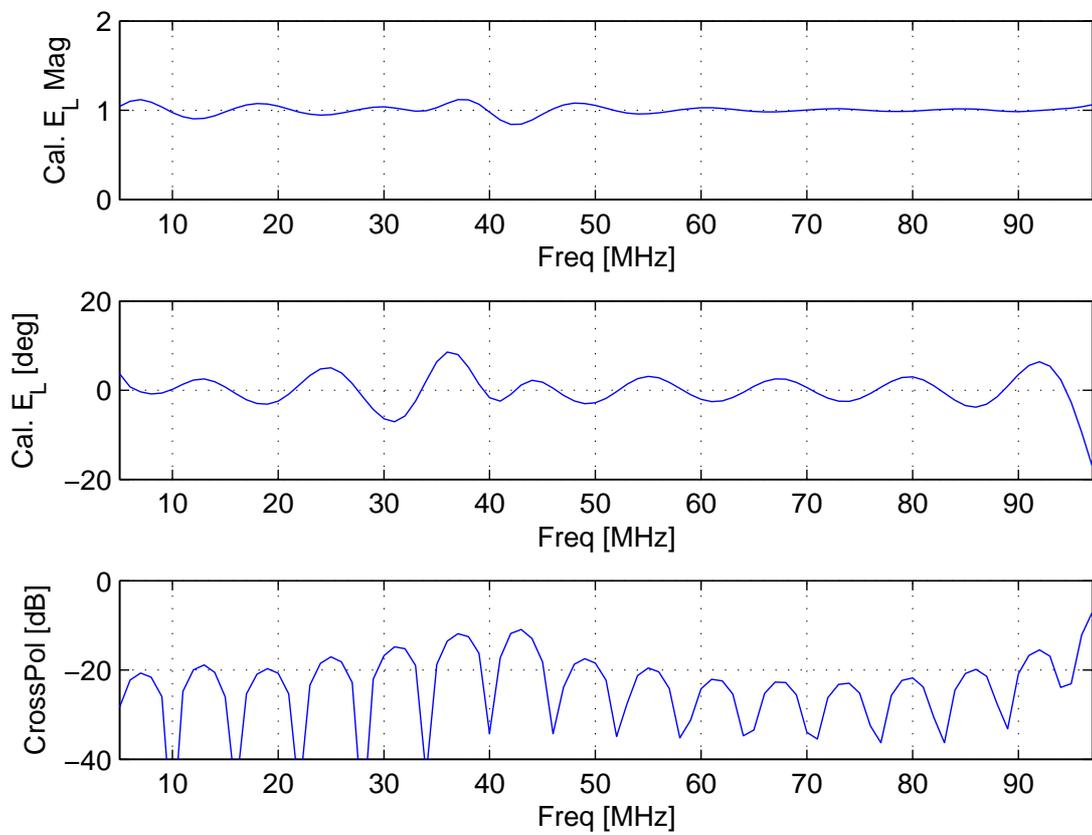
Figure 17:  $\theta = 74^\circ$ ,  $\phi = 0$ : Calibrated LCP using  $M = 16$  taps. Maximum tap dynamic range is 36 dB.
