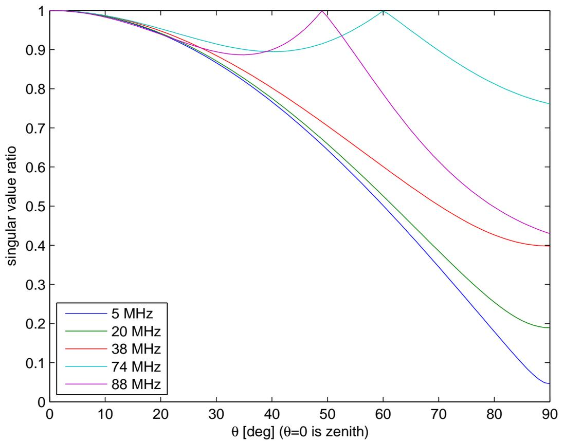
Figure 11: Efficacy of polarization calibration expressed in terms of singular value ratio; larger is better.  $\phi = 45^\circ$ .
