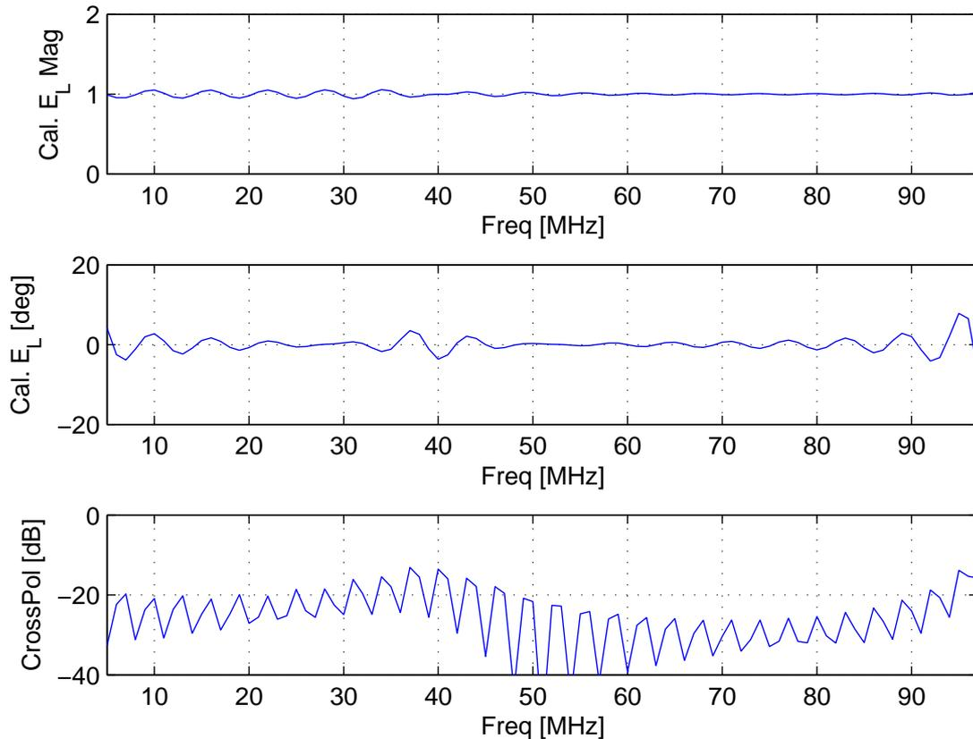
Figure 13:  $\theta = 74^\circ$ ,  $\phi = 45^\circ$ : Calibrated LCP using  $M = 32$  taps. Maximum tap dynamic range is 36 dB.
