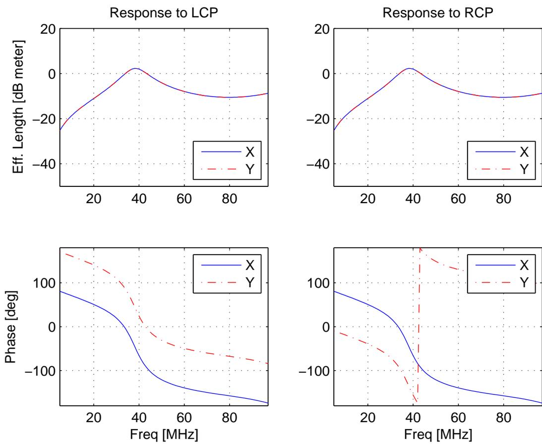
Figure 2: Zenith incidence: Active balun input.
