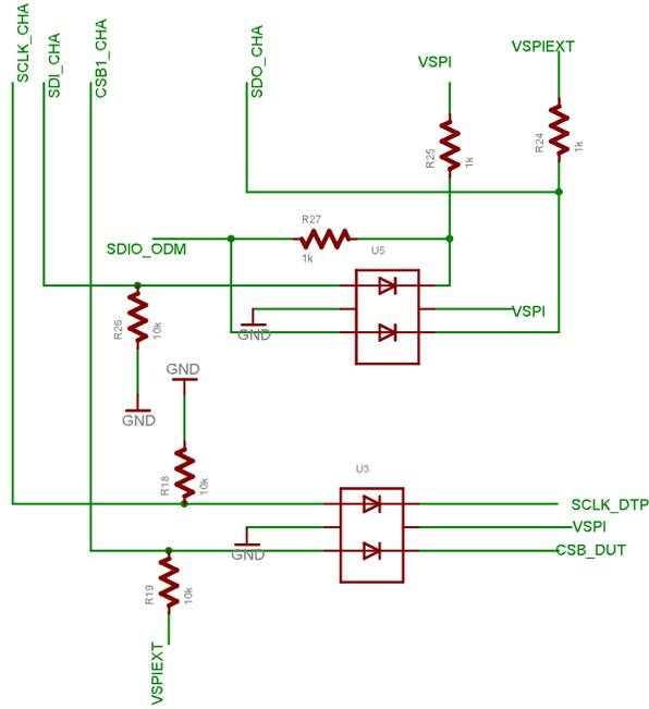
Figure 7: SPI circuitry. [Note. The resistors, capacitors, and inductors are reported in units of ohms, farads and henries respectively.]
