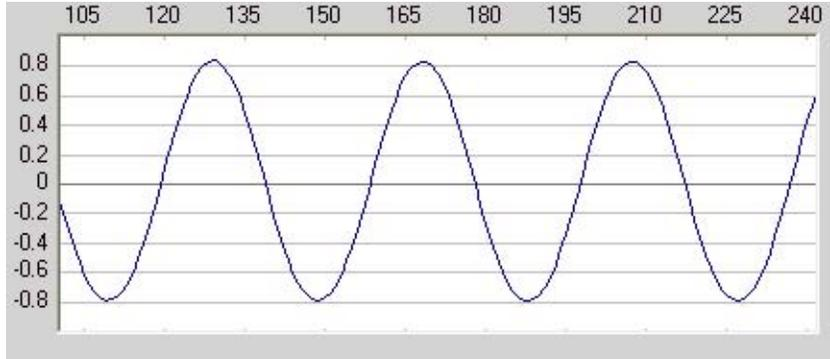
Figure 13: Time domain plot of few periods of a single tone at 5 MHz
