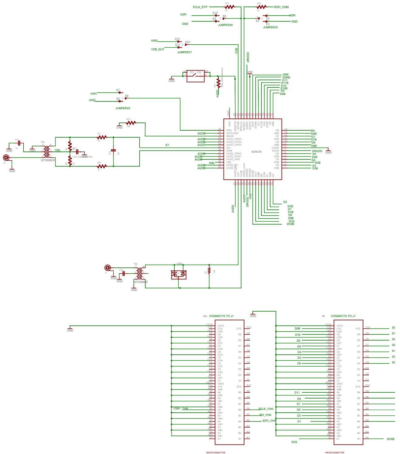
Figure 5: ADC circuitry. [Note. The resistors, capacitors, and inductors are reported in units of ohms, farads and henries respectively.]
