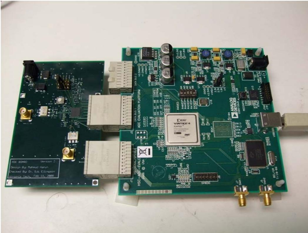
Figure 3: The VT prototype board connected to the Analog Devices HSC-ADC-EVALC board for evaluation.
