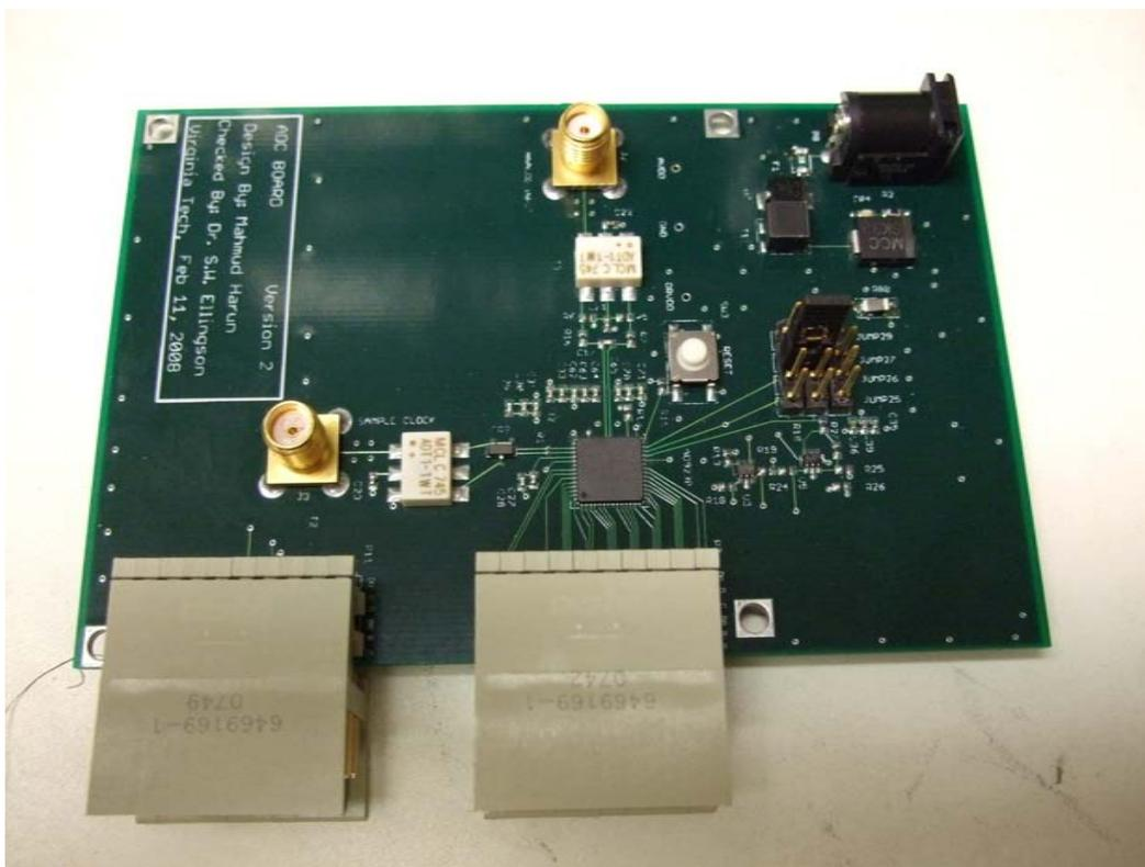
Figure 1: Top side of the VT prototype board.
