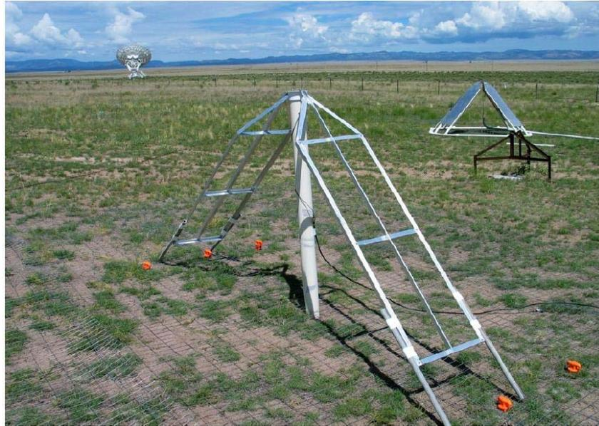
Figure 7 – Experimental Dipole Connected to G250R Balun
