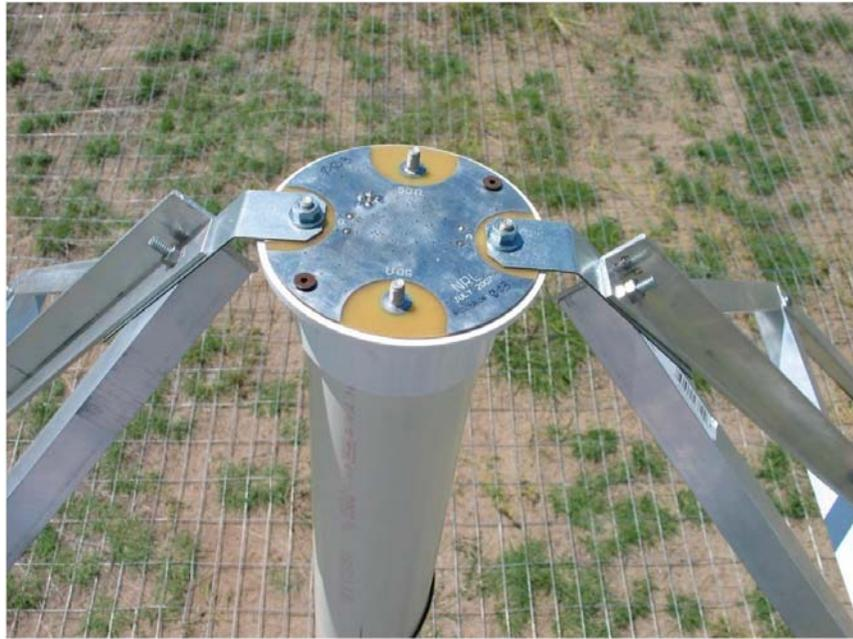
Figure 6 – Feedpoint Connections to G250R Balun
