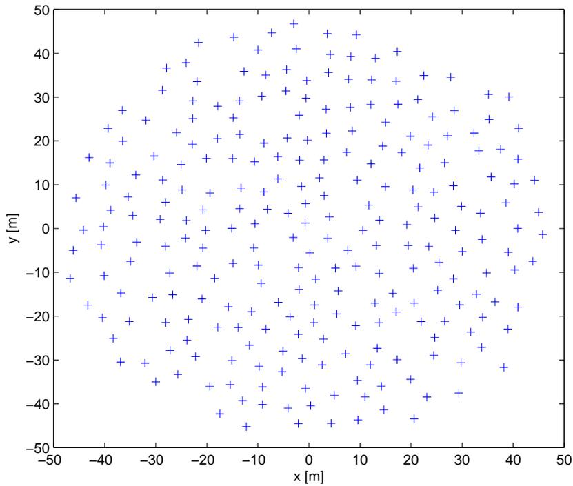
Figure 6: Candidate pseudorandom array geometry. *Courtesy A. Cohen, NRL.*
