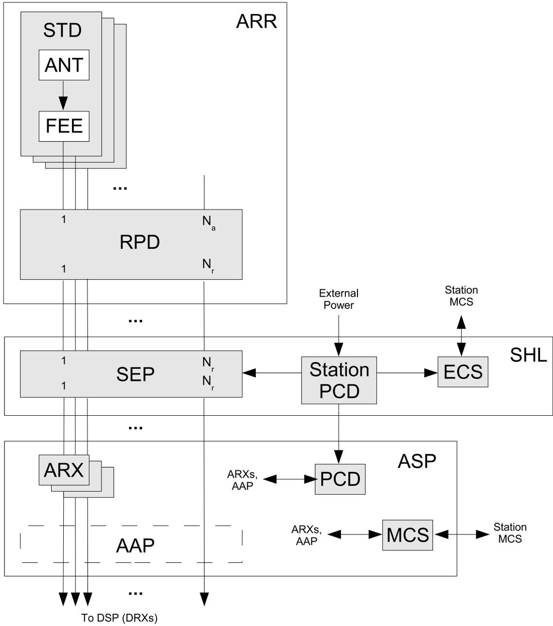
Figure 1: Station architecture: antennas through analog receivers.
