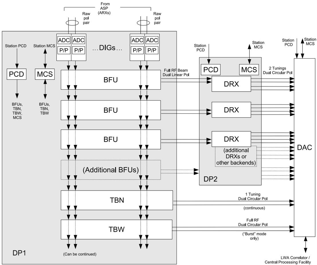
Figure 2: Station architecture: digital processing through external communications. The number of BFUs, TBWs, TBNs, and DRXs shown here may or may not represent the actual number used, and even at the time of construction and operation may not rigidly fixed; see the associated sections of this document for additional discussion. The DP1 daisy chain is explicitly shown, whereas the DP2 daisy chain(s) are not.
