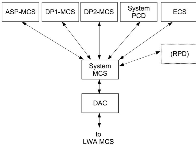
Figure 3: Station monitoring & control architecture. Interface to RPD is not necessary unless AAP is implemented there; see Section 3.3.
