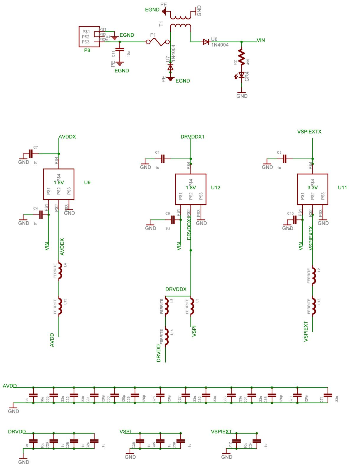
Figure 3: Power Distribution circuitry. [Note. The resistors, capacitors, and inductors are reported in units of ohms, farads and henries respectively.]
