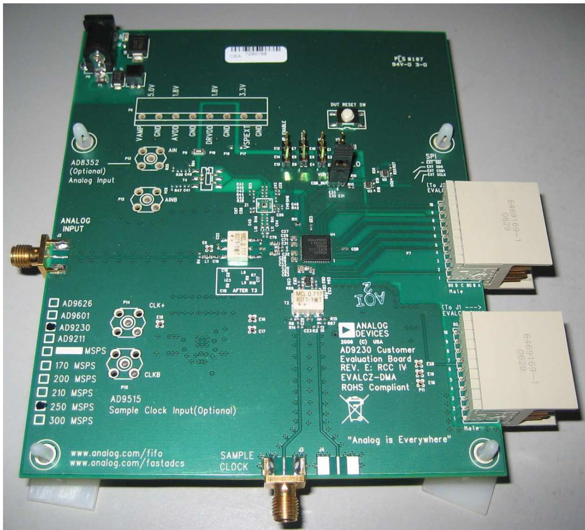
Figure 1: AD9230-250 Evaluation Board (Analog Devices Part No. AD9230-250EBZ)[3]. [Note. The AD9211-200 Evaluation Board is identical except for the A/D chip used.]
