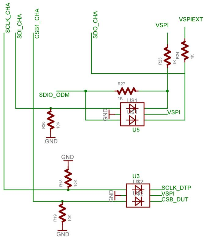
Figure 4: SPI circuitry. [Note. The resistors, capacitors, and inductors are reported in units of ohms, farads and henries respectively.]
