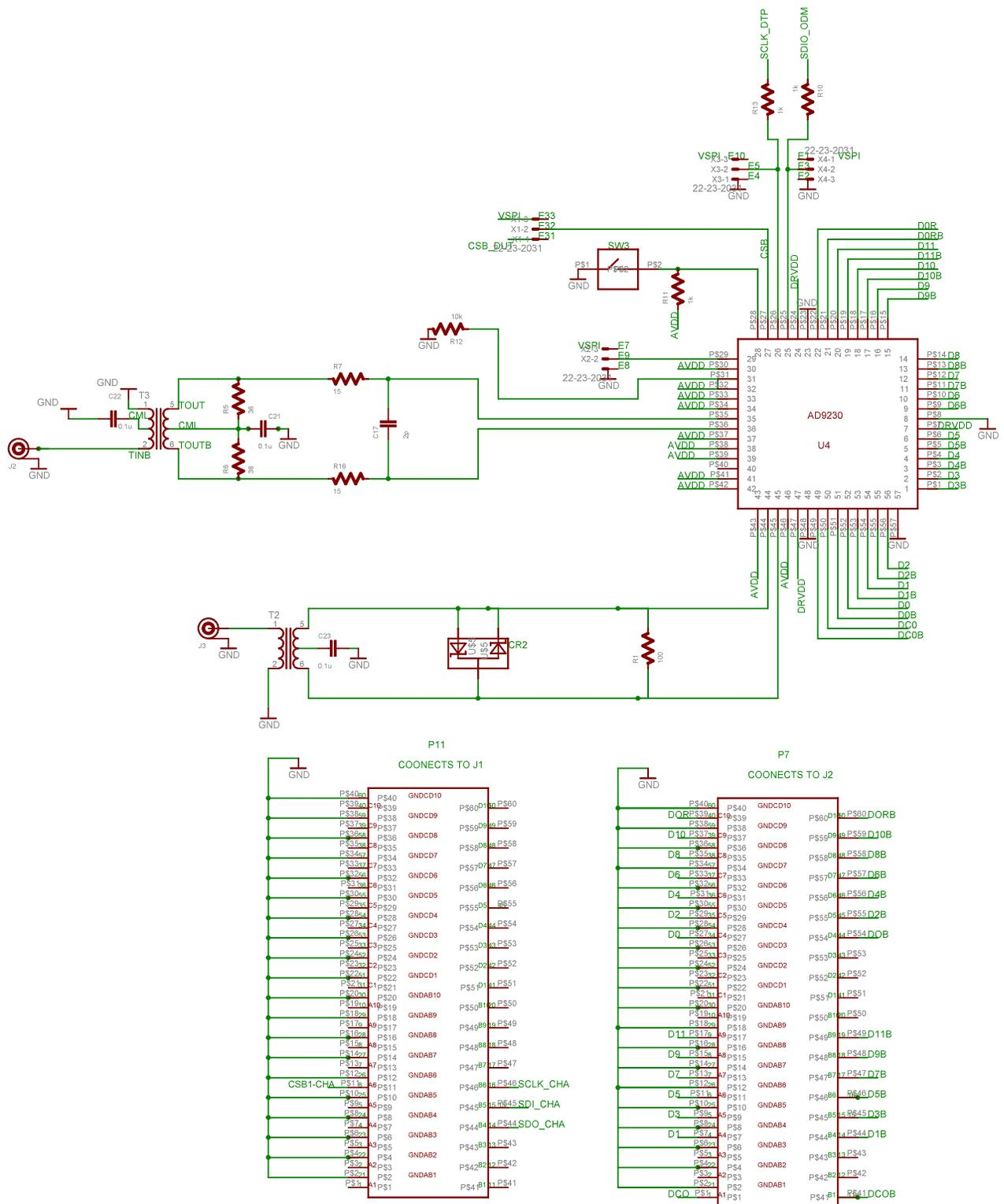
Figure 2: ADC circuitry. [Note. The resistors, capacitors, and inductors are reported in units of ohms, farads and henries respectively.]
