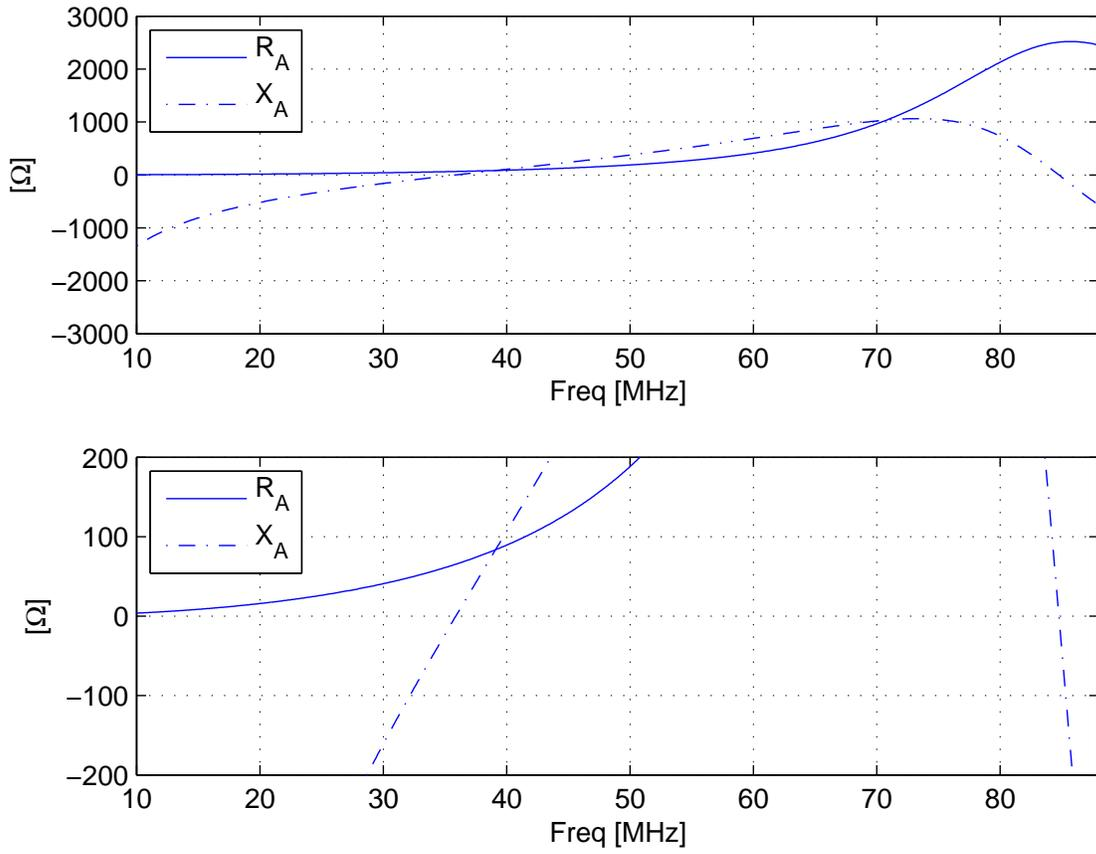
Figure 1: Impedance of a 4-meter-long straight dipole of radius 5 mm. The bottom panel is a close-up from the top panel.
