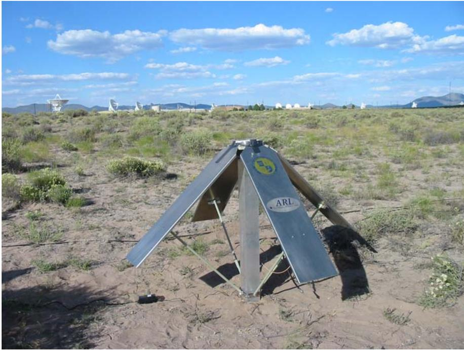
Fig. 1. Prototype blade antenna at the LWDA site.
